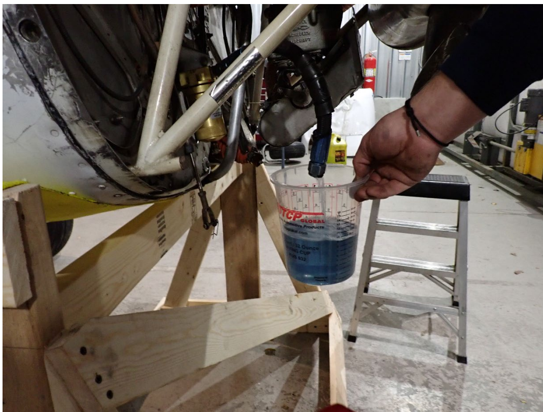
Figure 6 Fuel flow test carburetor fuel line
