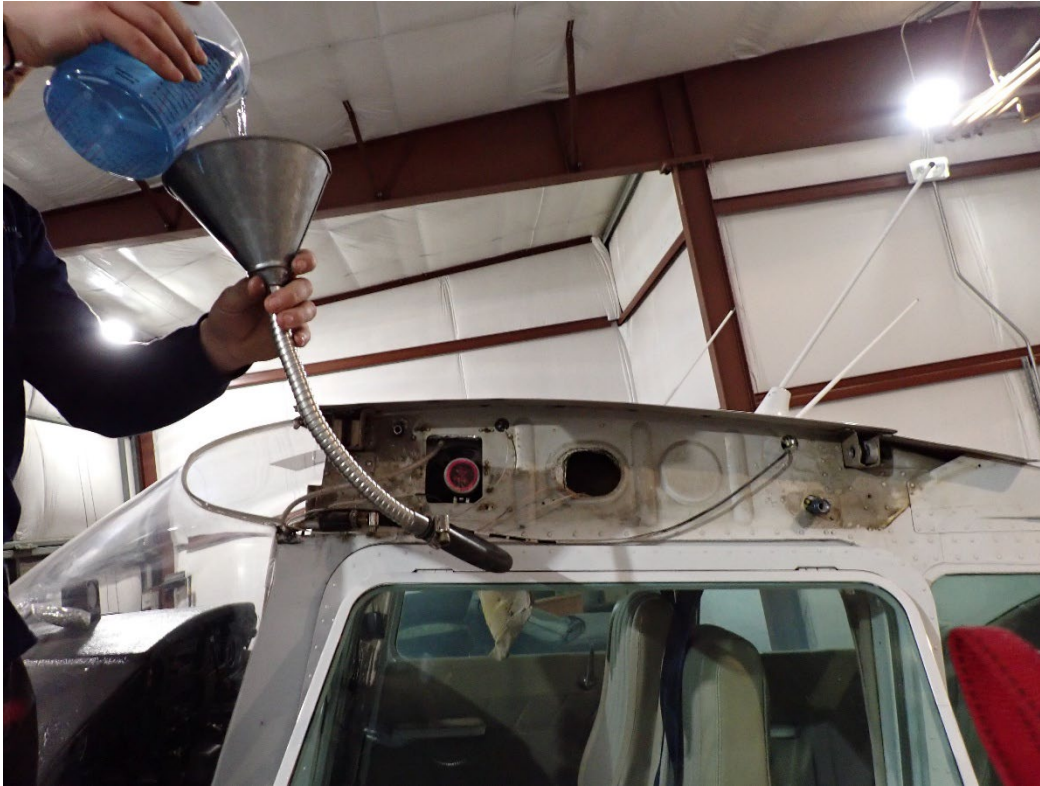
Figure 5 Fuel flow test with forward fuel line
