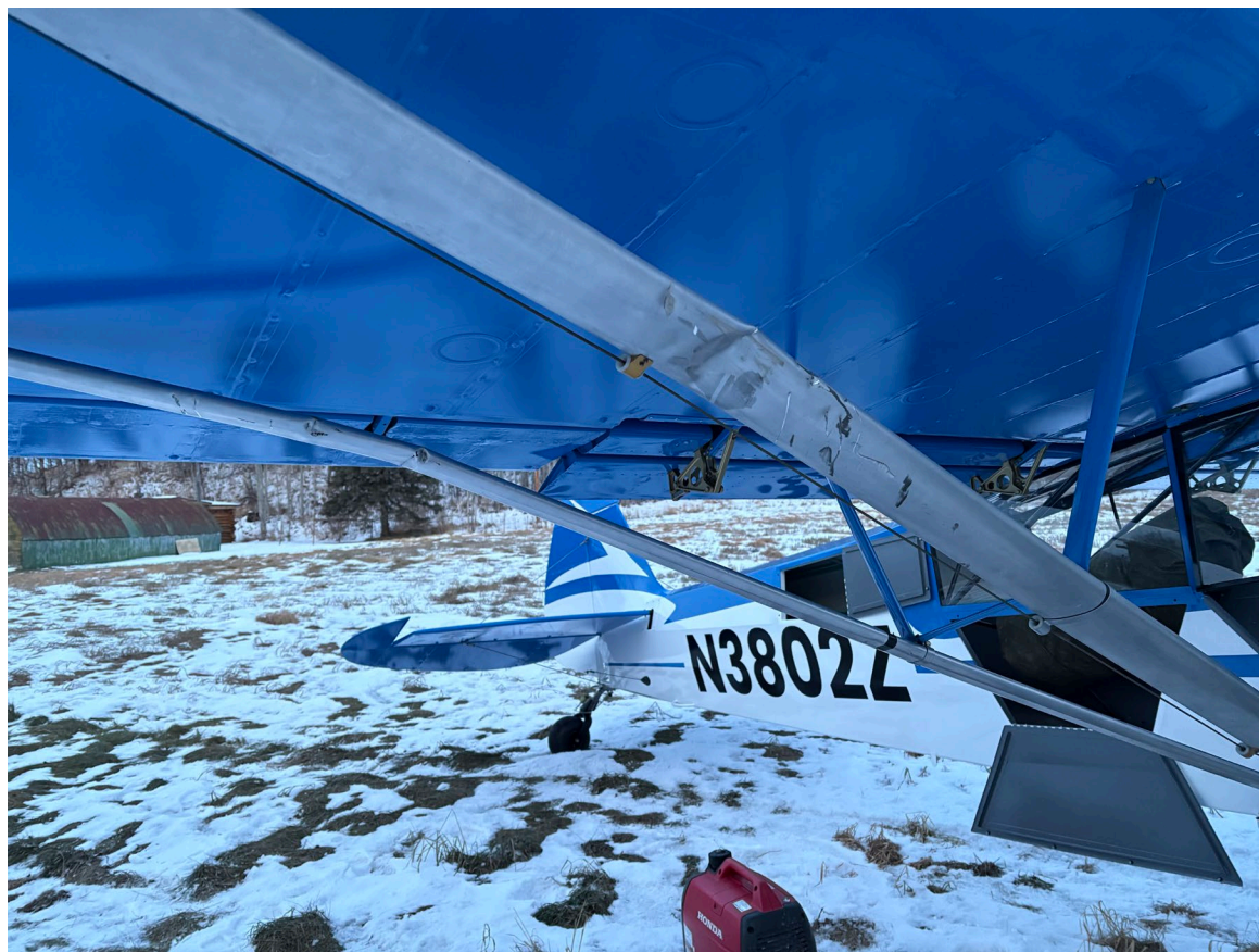
Photograph 2 - Damage to the right wing lift strut (Courtesy of owner)
