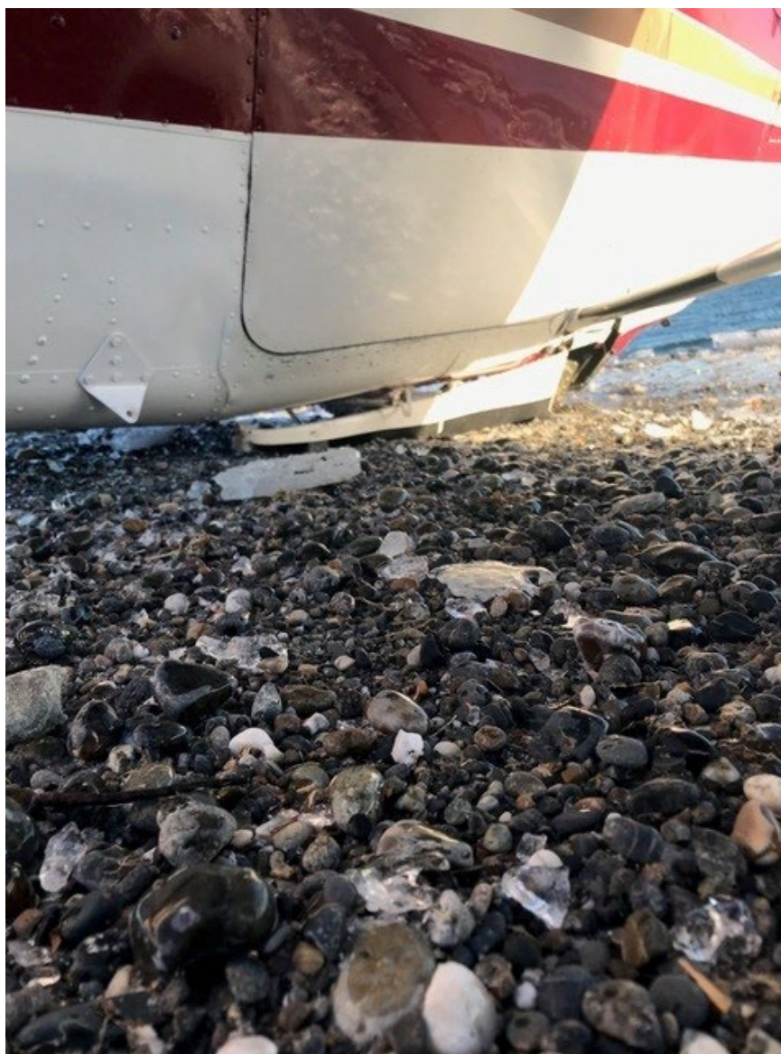
Photograph 2 - Right gear leg folded under fuselage (Courtesy of owner)
