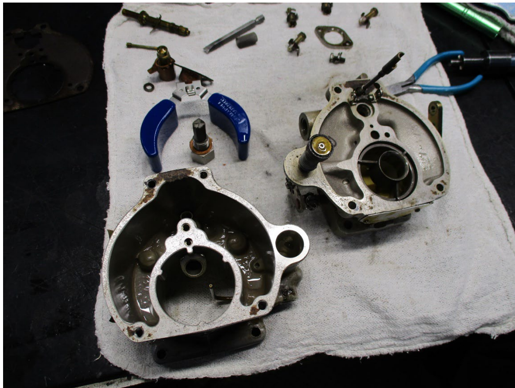
Figure 8 Carburetor disassembled at inspection
