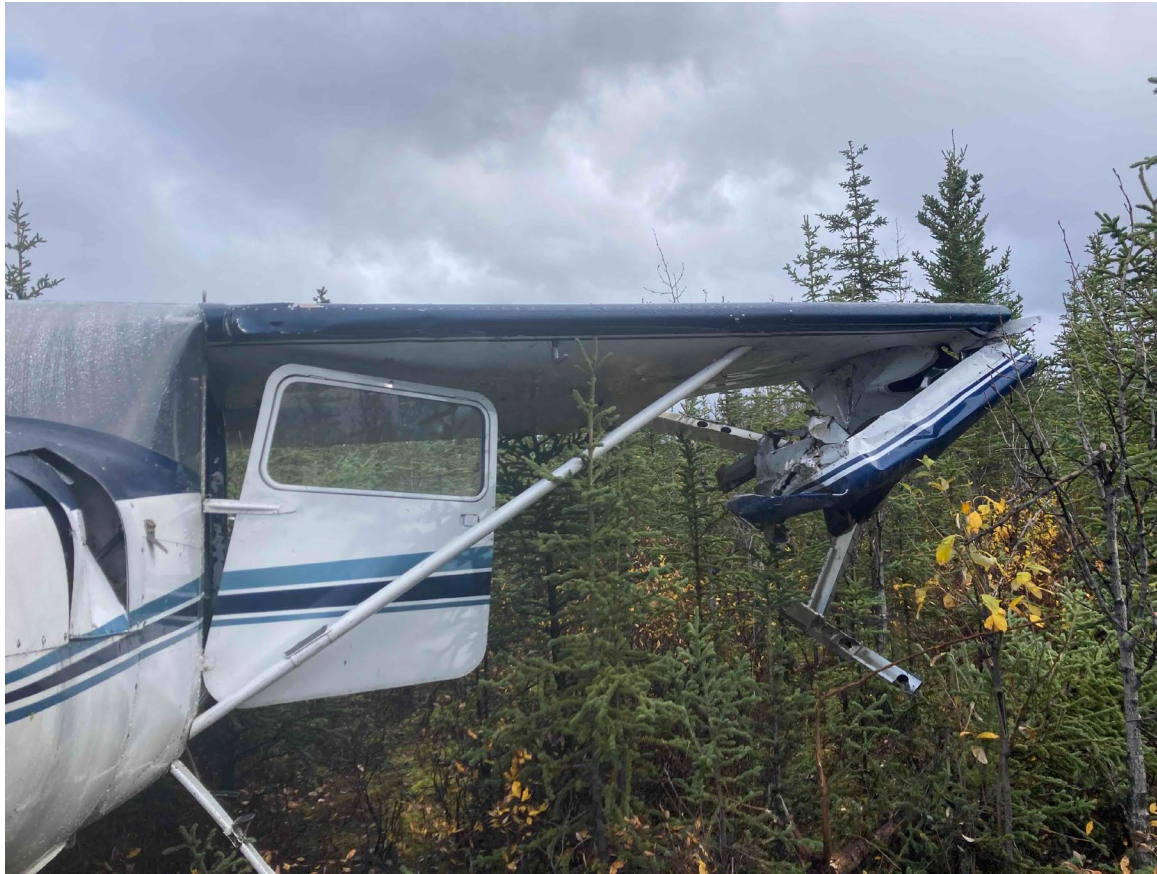
Photograph 2 - View of damage to the left wing (Courtesy of pilot)
