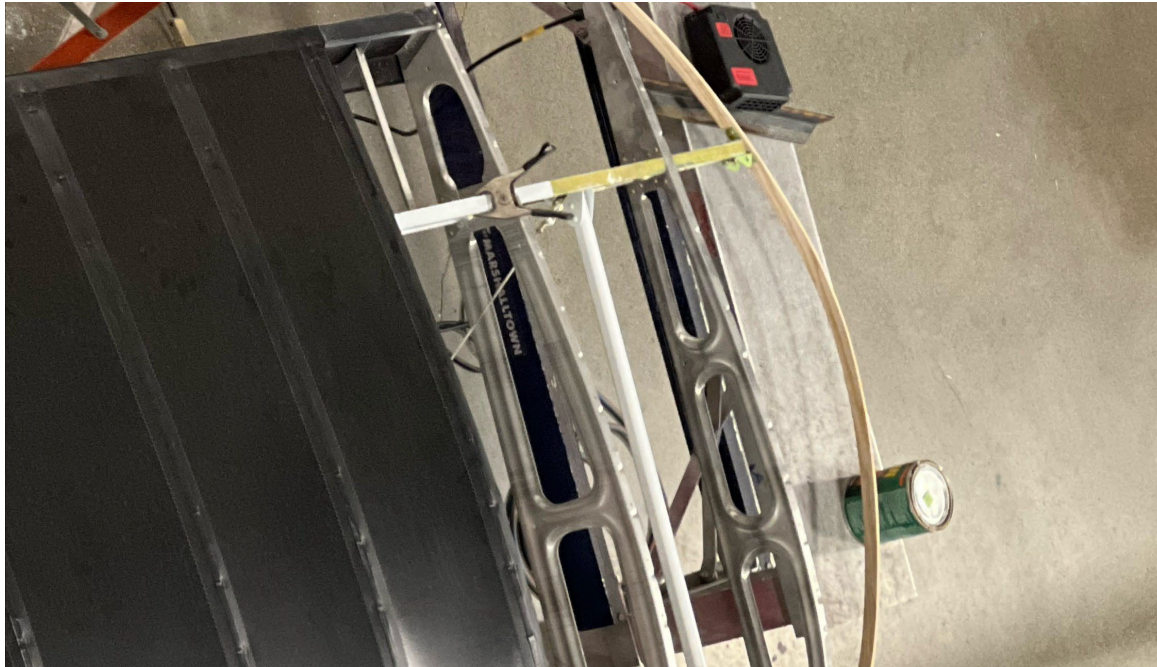
Photograph 1 - repair of spar and wing ribs (Courtesy of Owner)
