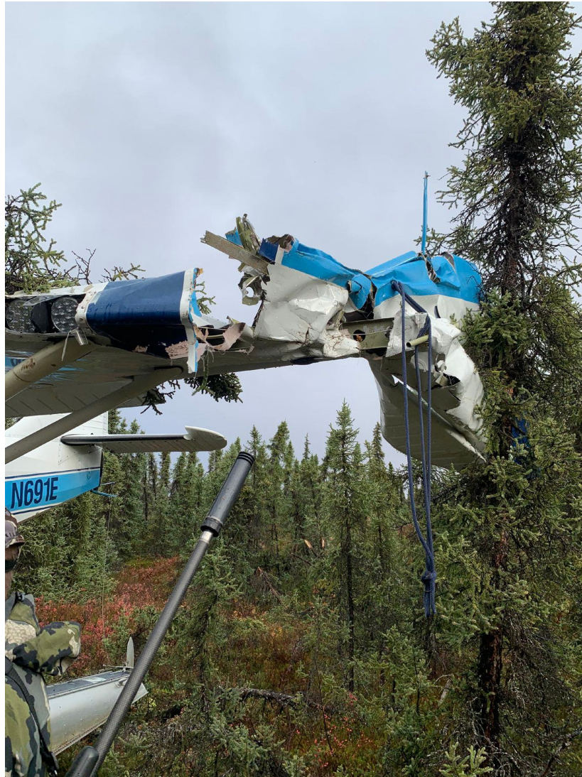
Photograph 2 - Left wing damage on accident airplane (Courtesy of owner)
