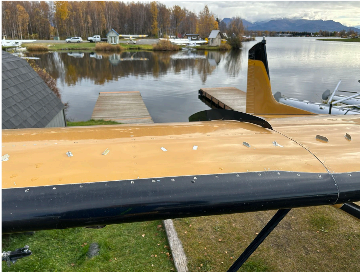
Photograph 2 - View of the top of the right wing missing vortex generators (Courtesy of FAA)
