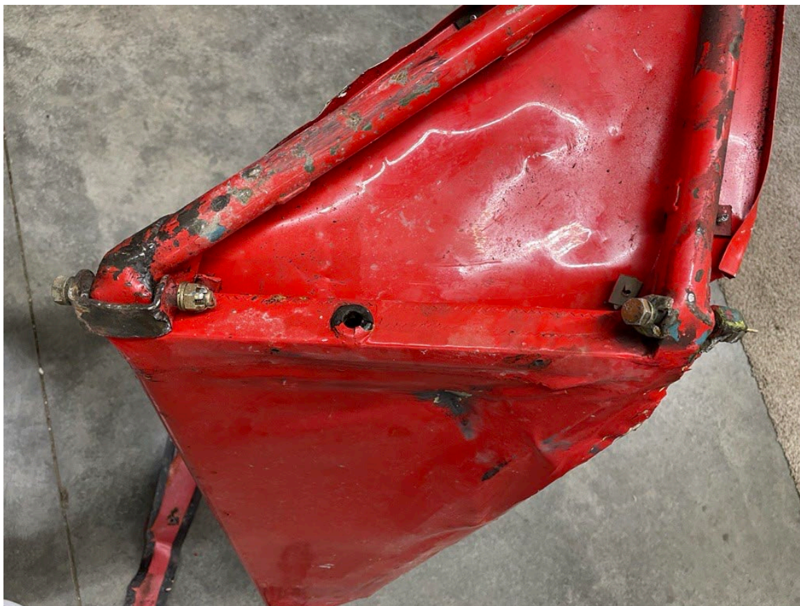
Photograph 3 - View of separated left main landing gear.
