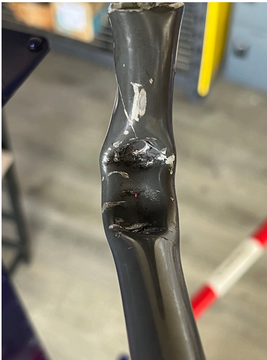
Photograph 4 - Push pull tube with witness signature from bolt (Courtesy of FAA)
