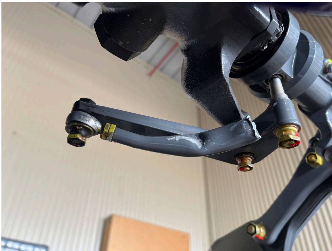
Photograph 1 - Push pull tube fractured at bell crank (Courtesy of FAA)
