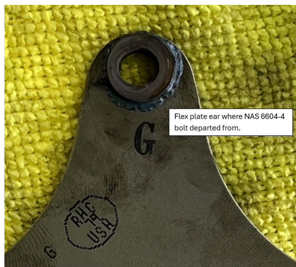
Figure 7 Ear of aft flex plate with wear signature
