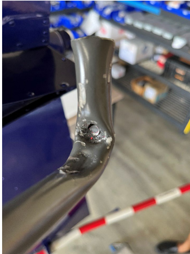
Figure 3 Tail rotor push pull tube with witness signature from bolt.
