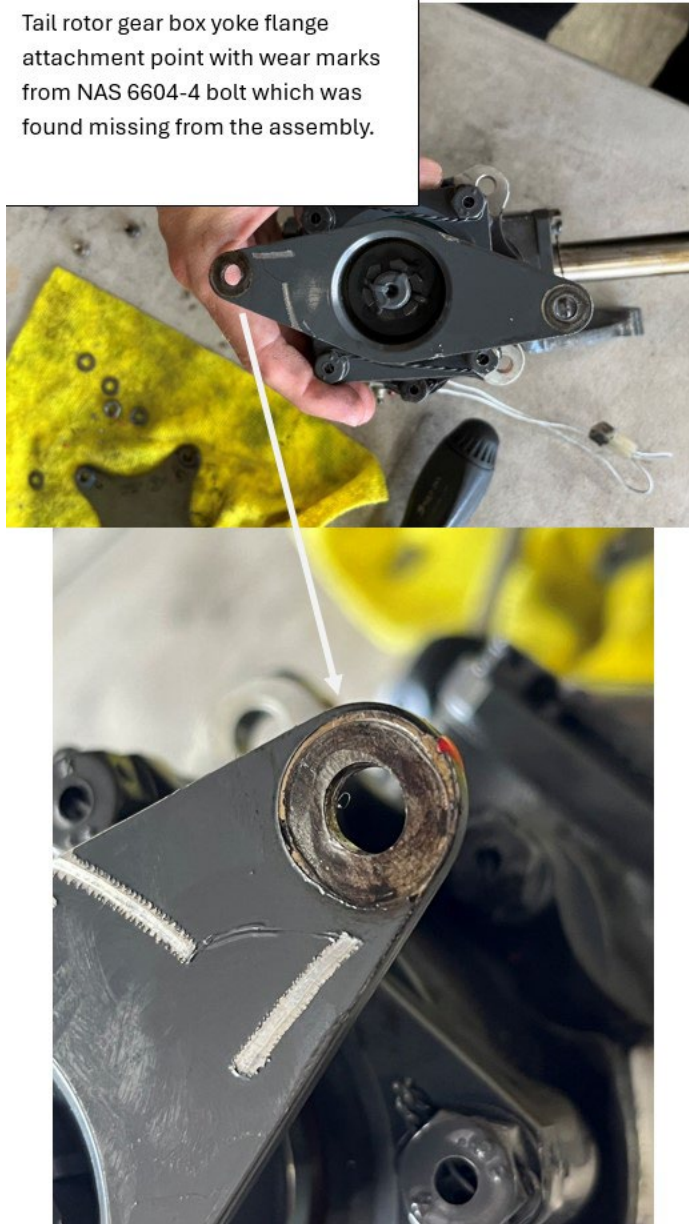
Figure 8 Tail rotor drive shaft yoke flange
