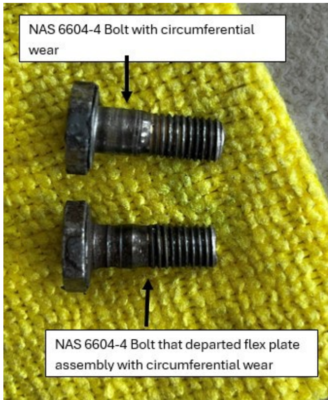
Figure 4 NAS 6604-4 bolts with circumferential wear
