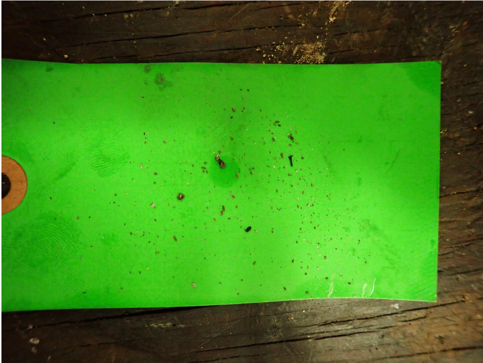
Figure 13 Debris found in carburetor
