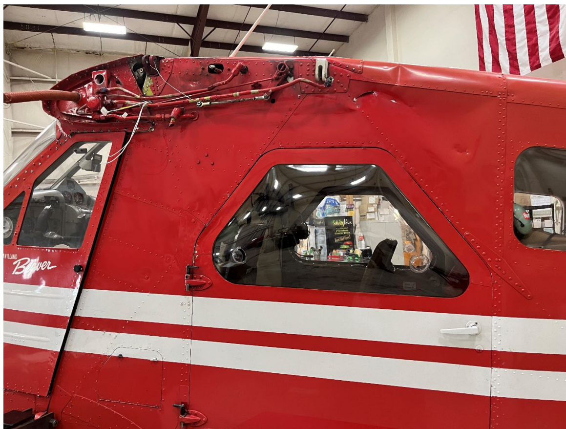
Photograph 2 - Damage to wing root attachment point
