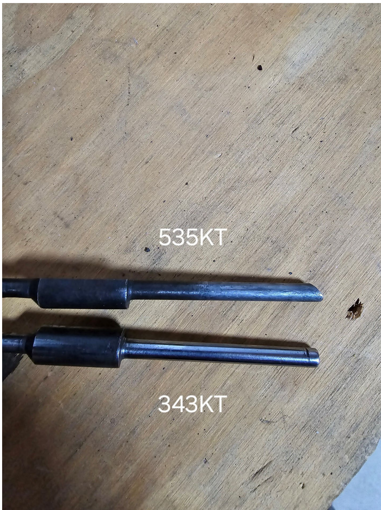
Figure 6 View of bent cam compared to an undamaged cam rod.
