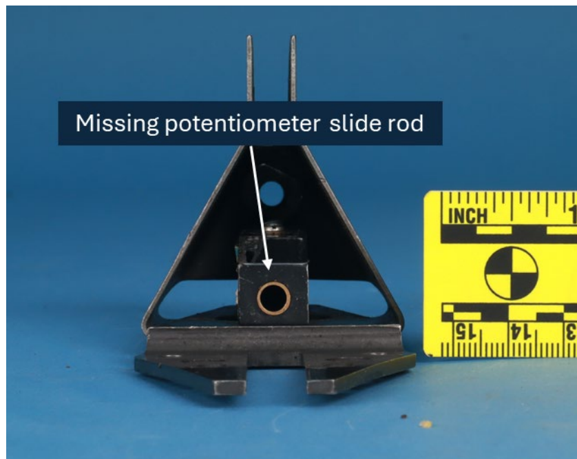
Figure 10. The potentiometer slide rod was not recovered.
