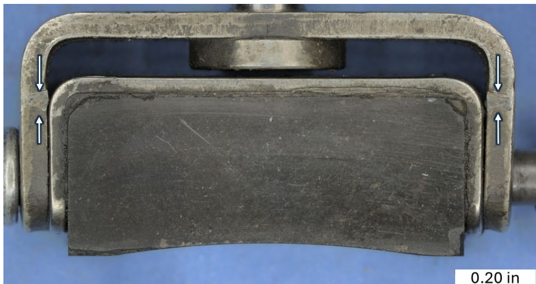
Figure 6. The carbon block and yoke. White arrows indicate grooves found on the yoke.
