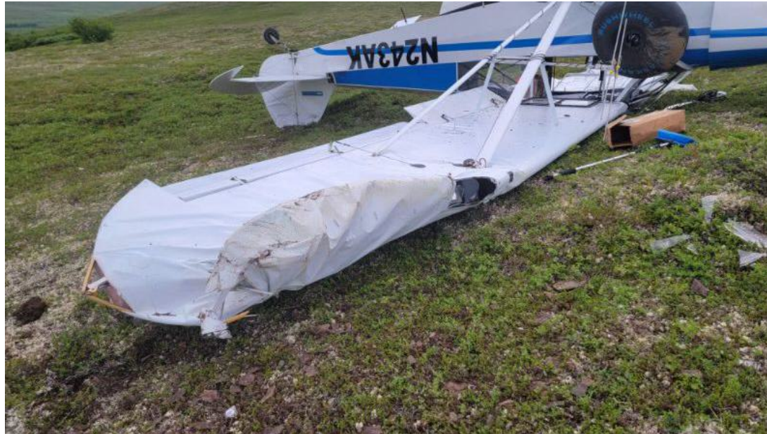
Photograph 3 - View of Damage to left wing (Courtesy of Pilot)
