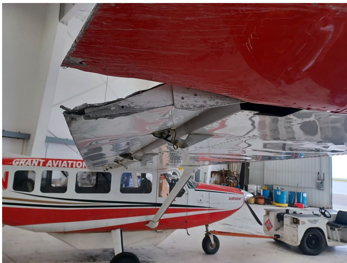
Photograph 1 - View of damage to the bottom of the wing and aileron (Courtesy of operator)
