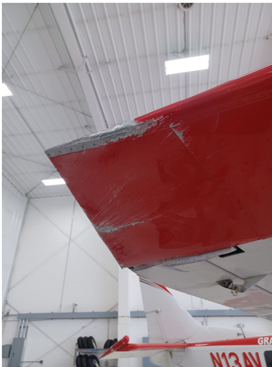
Photograph 3 - View of wingtip damage (Courtesy of operator)
