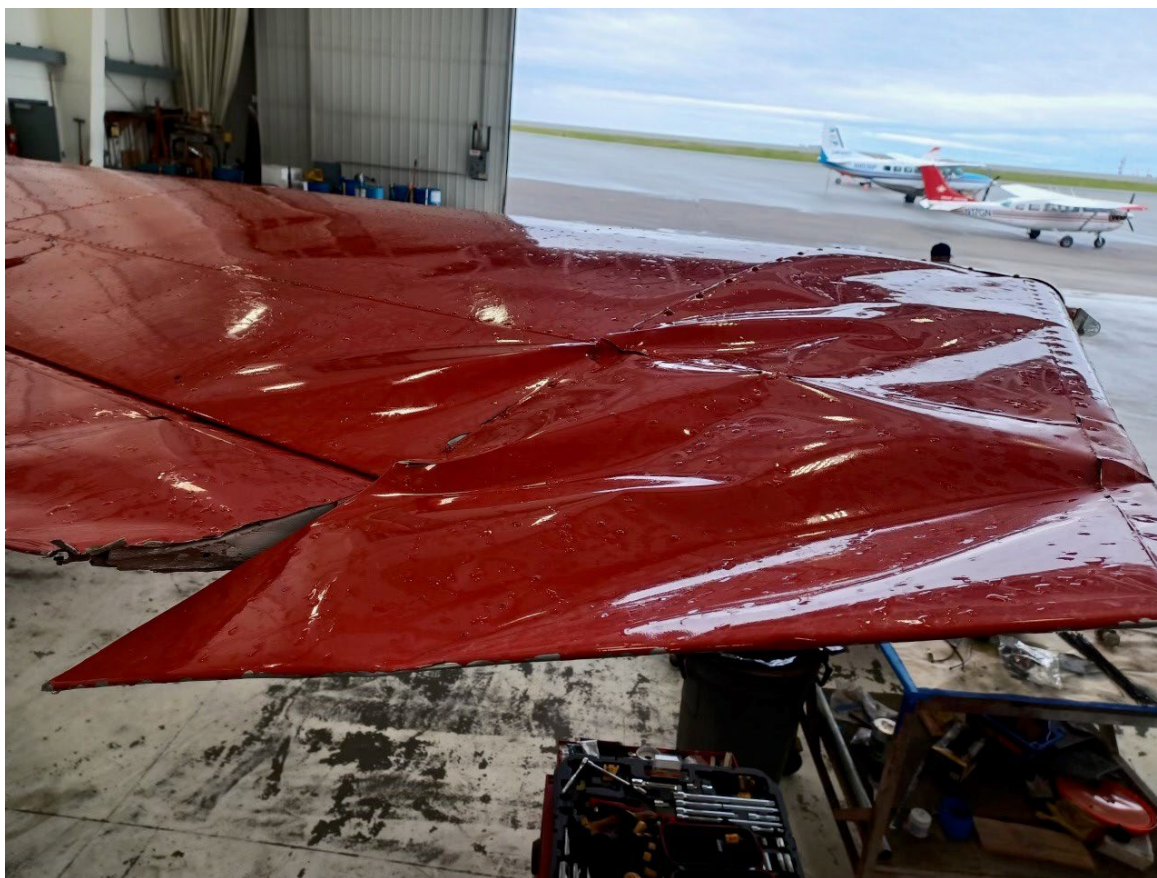
Photograph 2 - View of damage to the top of the wing (Courtesy of operator)
