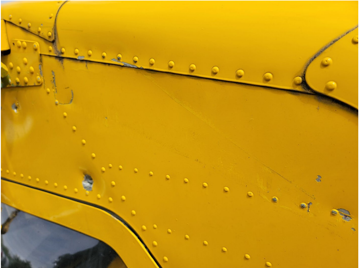
Figure 3 View of witness mark left by left side flap during impact.
