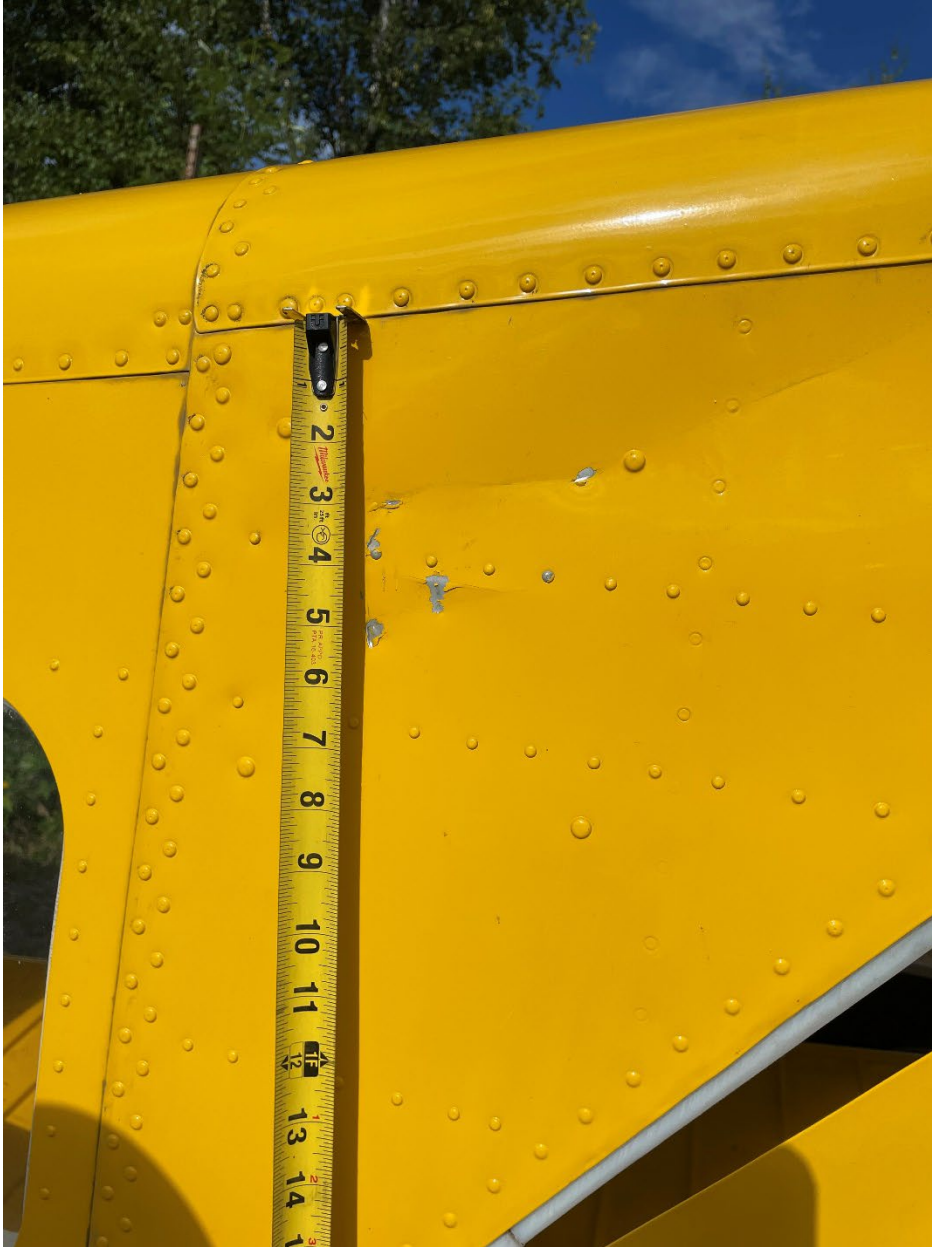
Figure 2. View of witness mark left by right side flap during impact.
