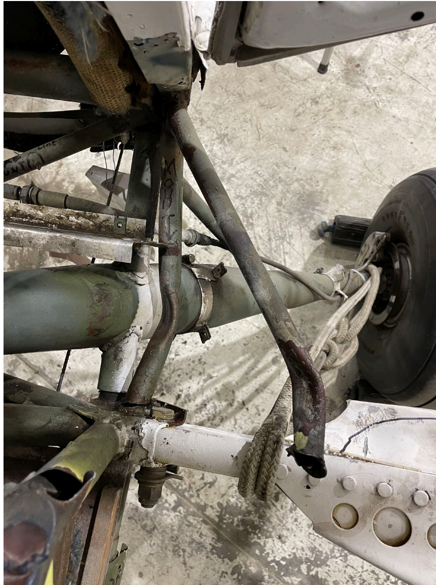
Photograph 2 - View of the damage to the fuselage.
