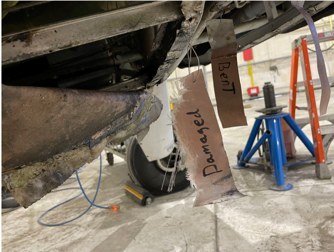
Photograph 3 - View of damage to the bottom of the fuselage.
