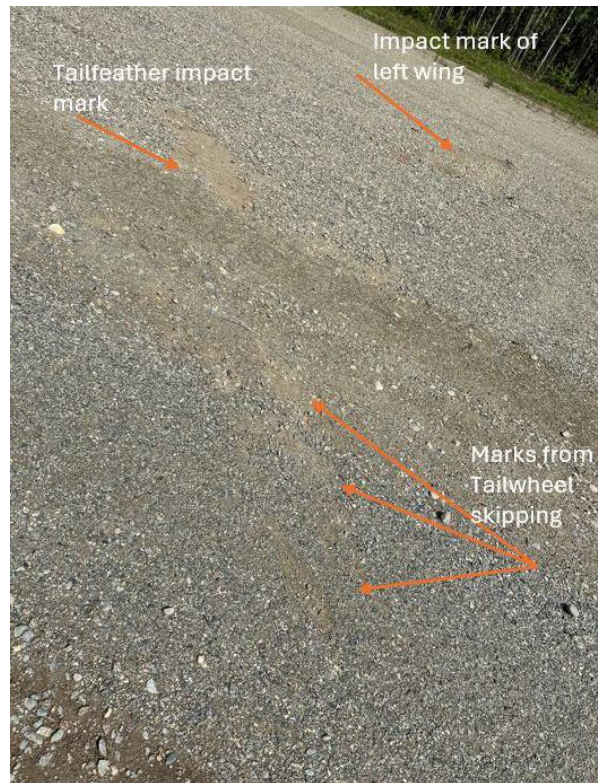
Figure 3 Impact marks from tailwheel
