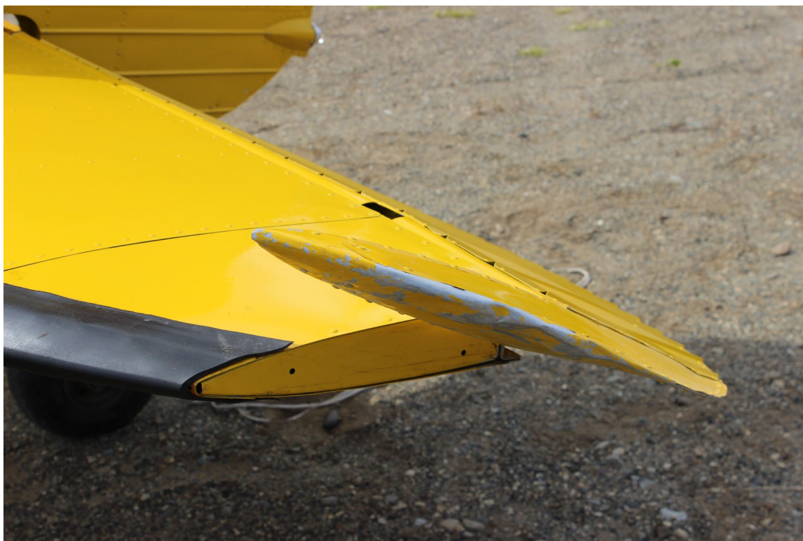
Photograph 3 - Damage to left elevator
