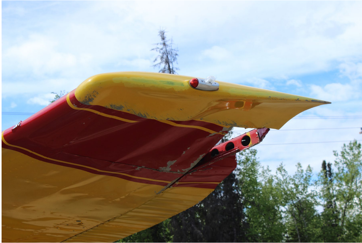
Photograph 2 - Damage to left wing tip
