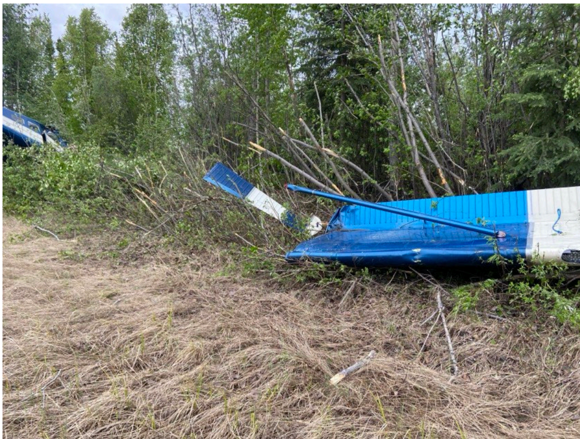
Photograph 2 - Image of liberated right wing and right elevator (Courtesy of Pilot)
