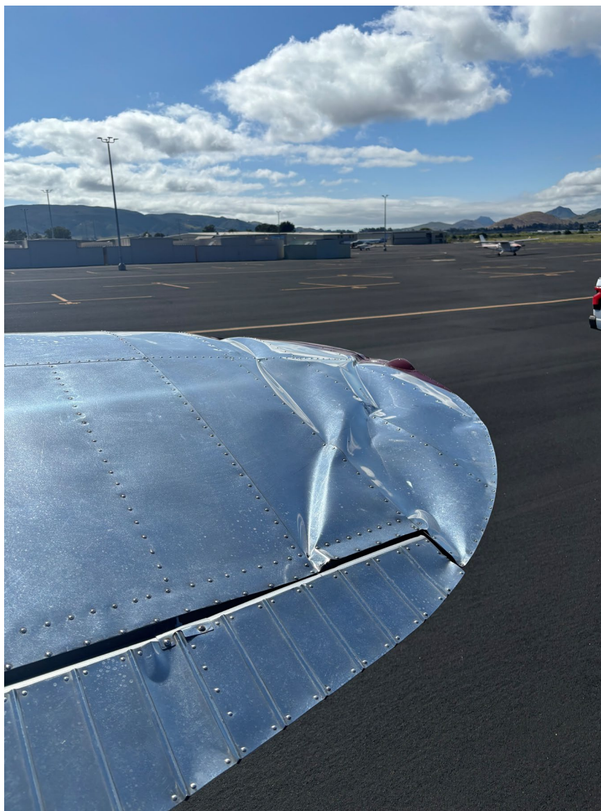
Photograph 2 - Image of damaged right wingtip and aileron (Courtesy of Airport Operations)
