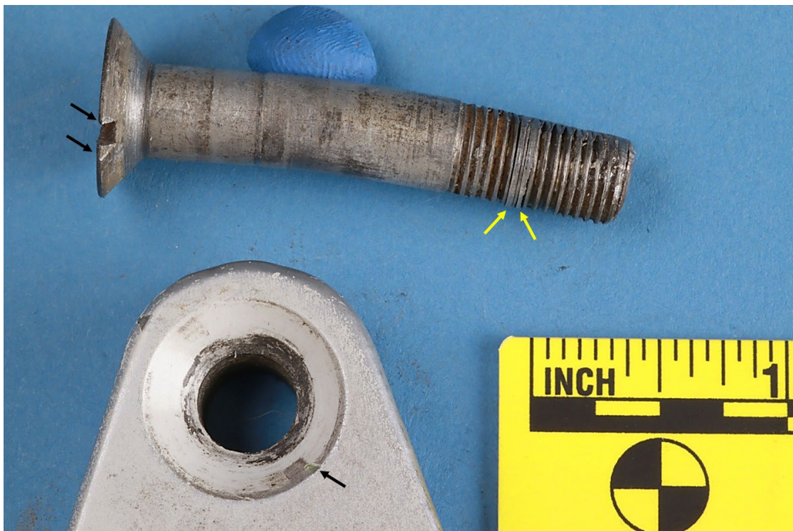
Figure 6. Photograph of the countersunk attachment bolt relative to the countersink in the axle. Witness marks on the fastener aligned with chipped paint on the axle. Fragments of metal were retained in the fastener threads as indicated by yellow arrows.
