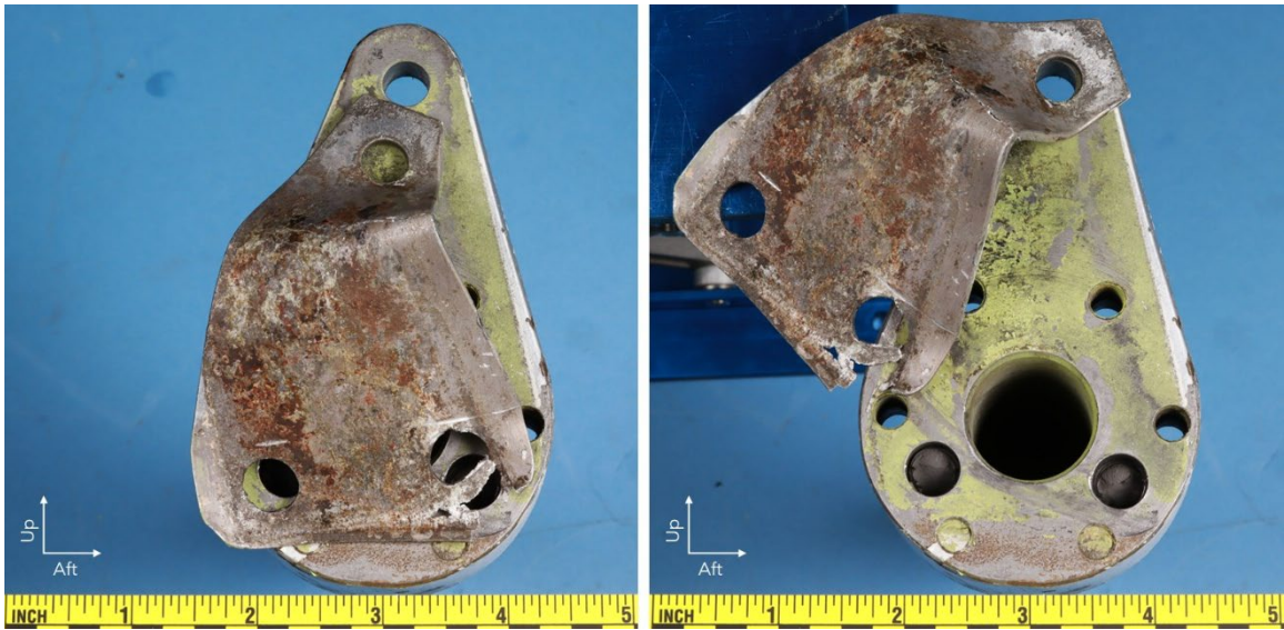
Figure 5. Photographs of the tapered shim aligned with the bottom fastener holes (left) and the top fastener hole (right) relative to a curved witness mark where the primer had been scraped away.
