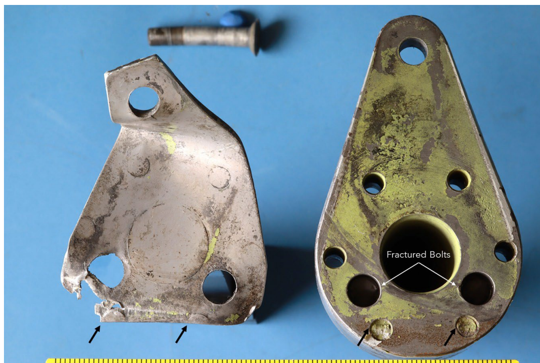
Figure 2. Photograph of the mating surfaces of the tapered shim (left) and axle (right). Corresponding witness marks are indicated by black arrows.
