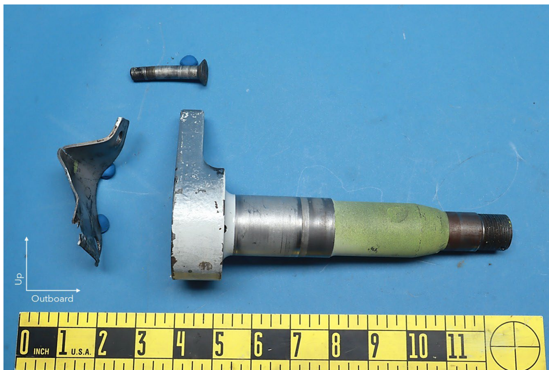
Figure 1. Photograph of the axle (right), tapered shim (left), and countersunk bolt (above) as received.
