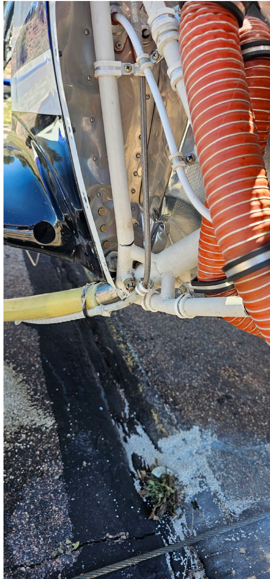
Photograph 2 - Image of fractured engine mount tubing (Courtesy of Operator)
