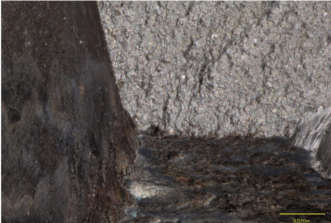
Figure 11. Angled view of the piston initiation area.
