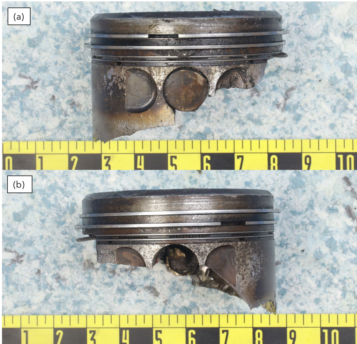
Figure 3. Side views of the piston from the pin boss sides showing (a) the side with the cap still in place and (b) the reverse side.
