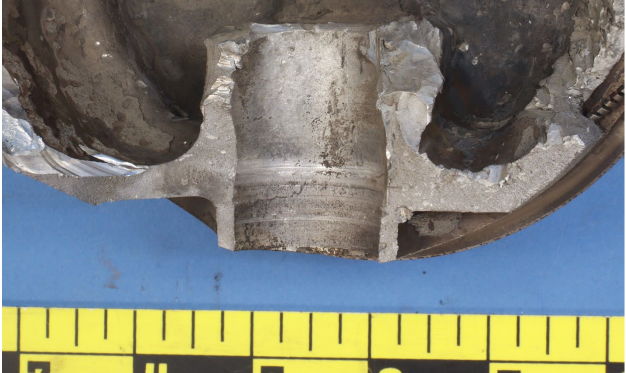
Figure 5. View of the fracture surface near the pin on the piston.
