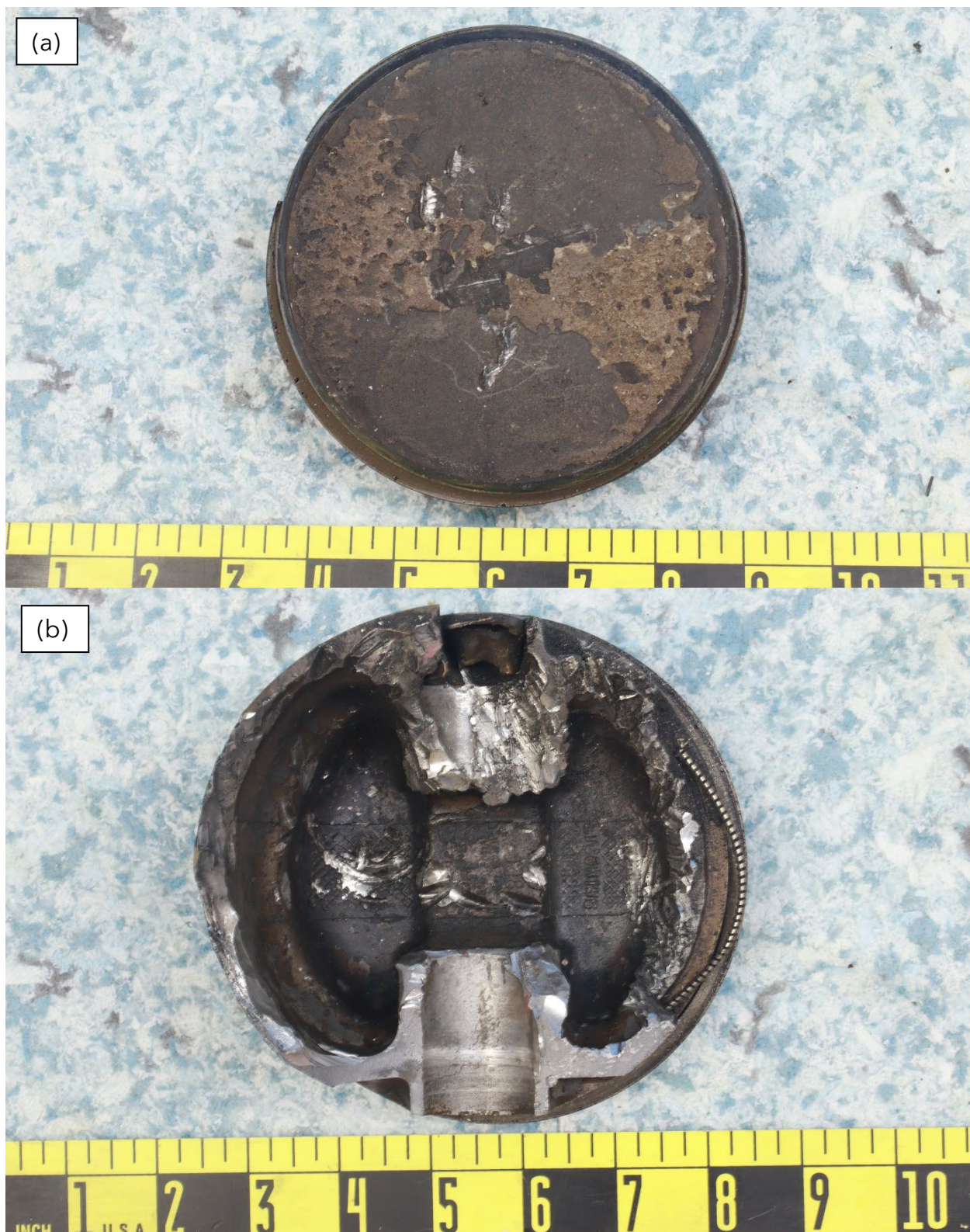
Figure 2. Views of the piston remnant from (a) the crown and (b) the underside and skirt, as received.
