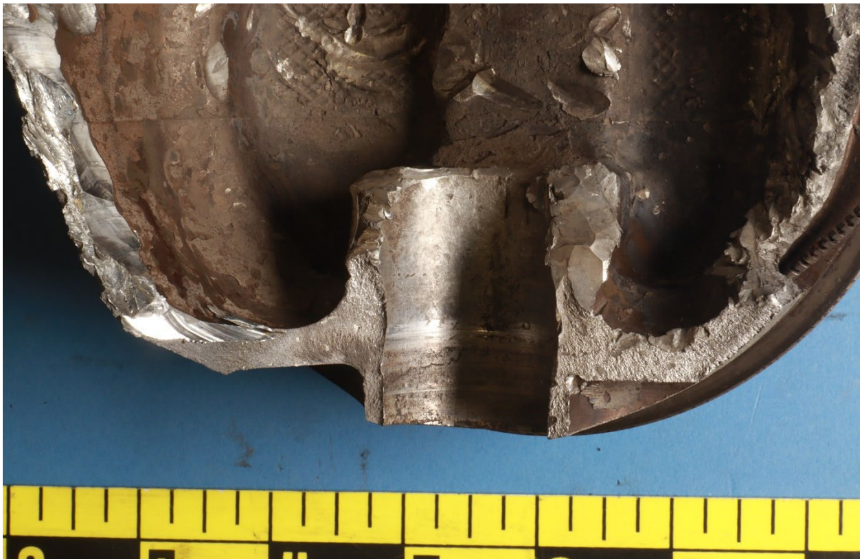
Figure 6. Oblique lighting view of the piston fracture surface in Figure 5.
