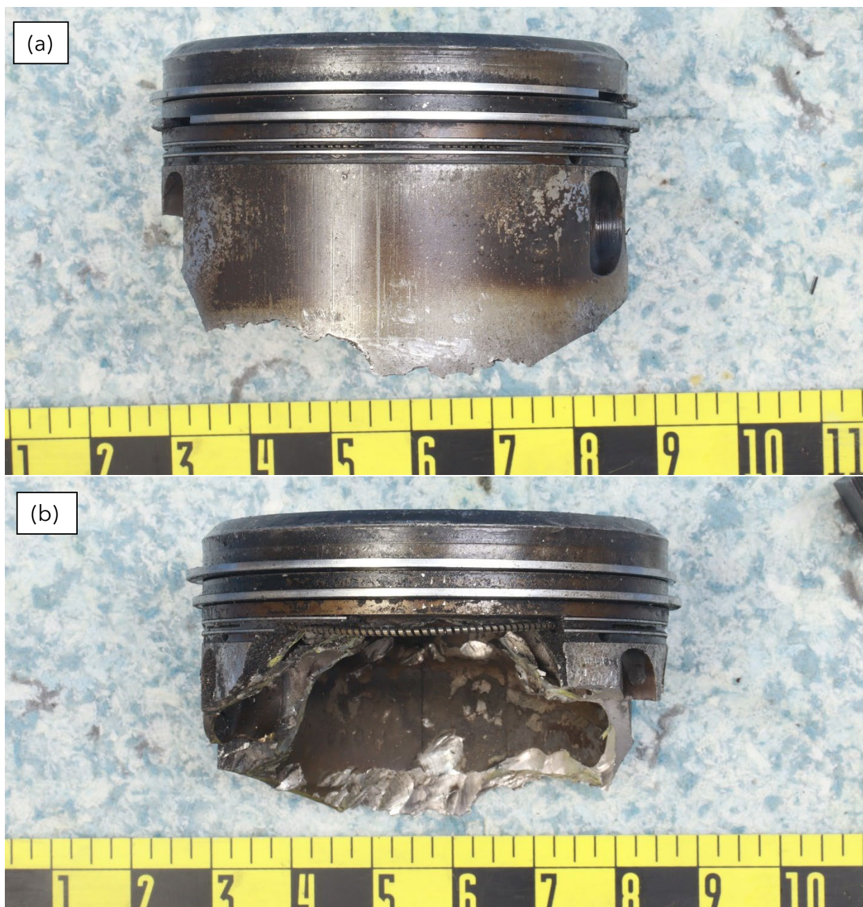
Figure 4. Side views of the piston remnant from (a) the longer skirt remnant side and (b) the short side, as received.
