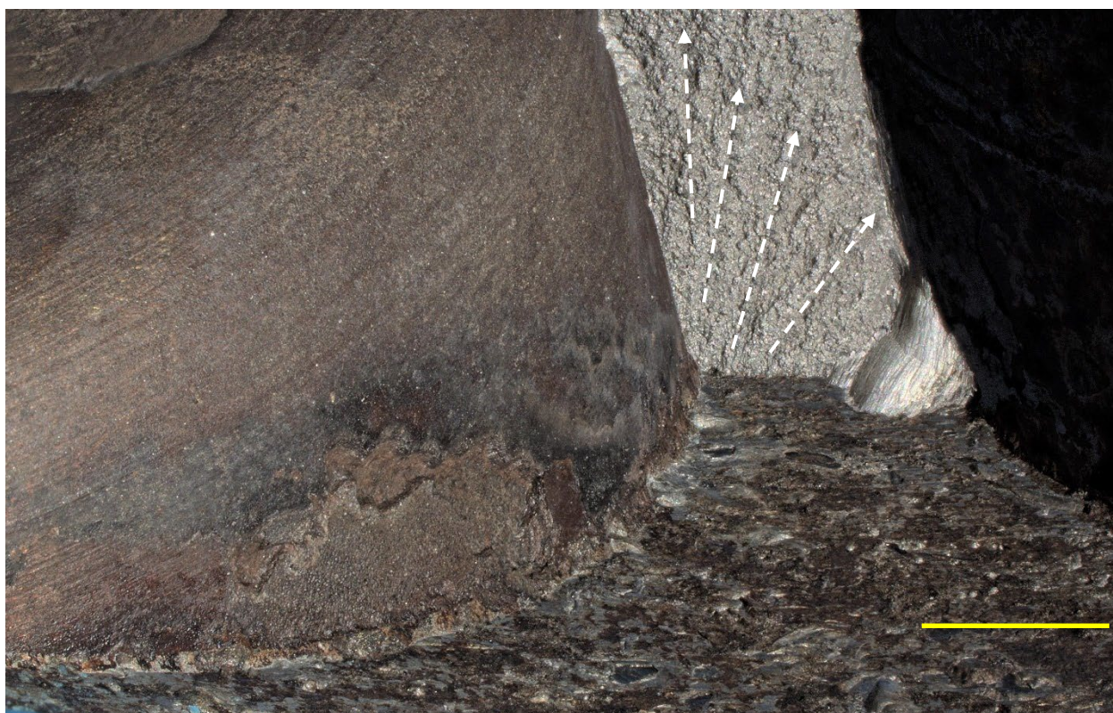
Figure 10. Angled view of the piston initiation area, annotated to show the fracture direction.
