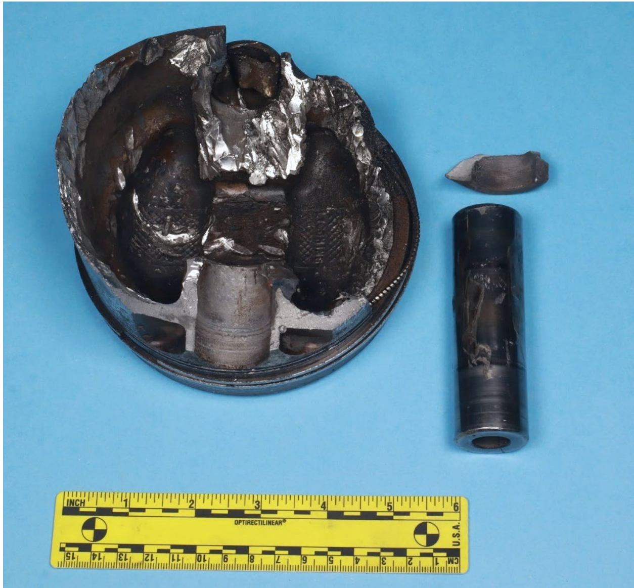
Figure 1. The pieces submitted from the accident, the piston remnants and the piston pin.
