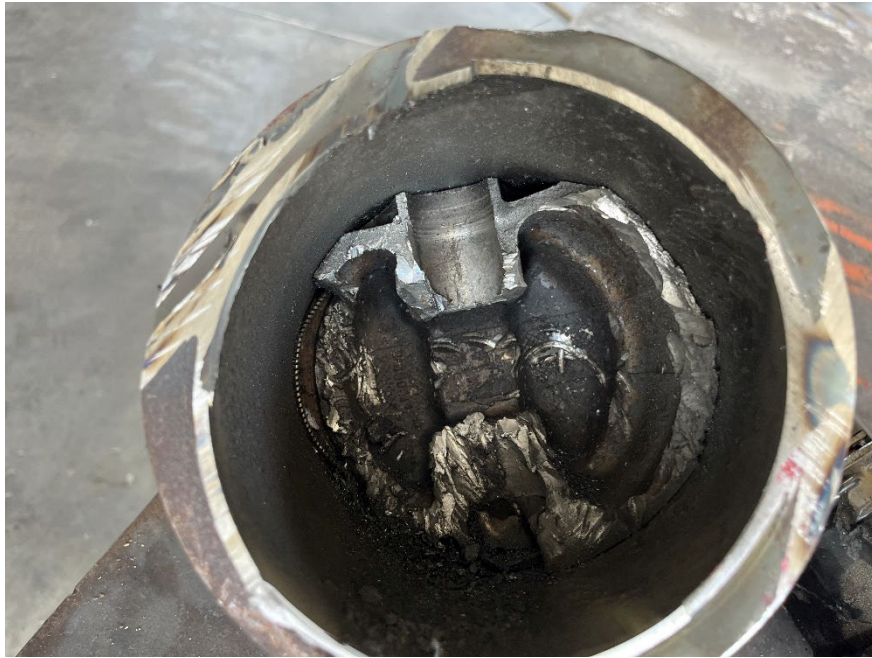
Figure 6 Cylinder #4 piston skirt and wrist pin boss damage
