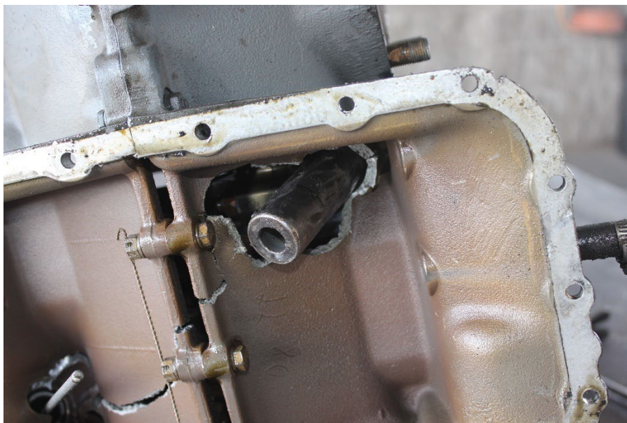
Figure 5 Wrist pin embedded in lower crank case
