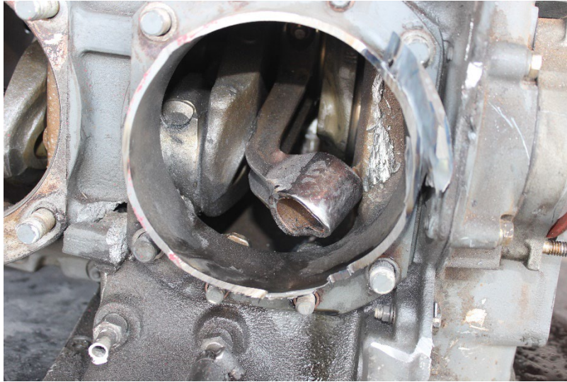
Figure 4 Bent Connecting Rod #4 Cylinder
