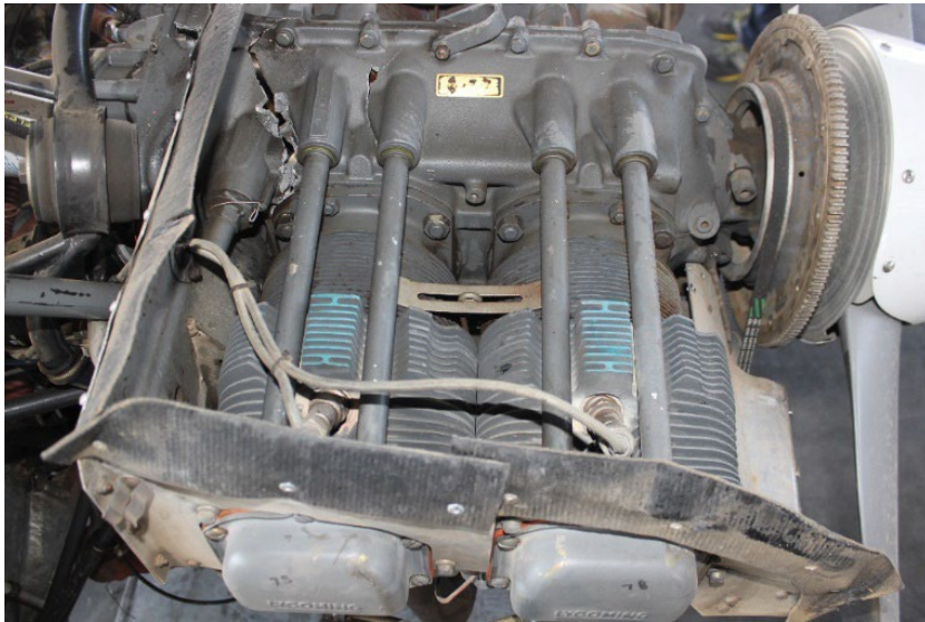
Figure 2 Crack in crank case beginning near the top of cylinder #3
