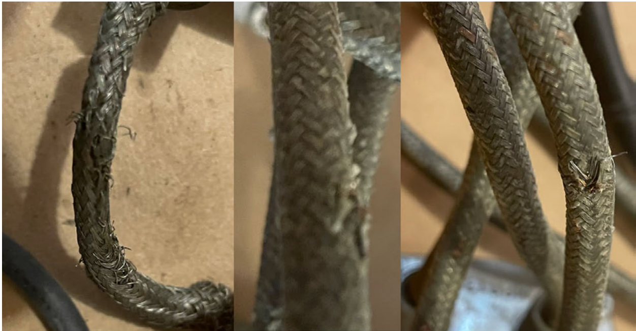
Figure 14 View of damage to the high-tension sparkplug lead wires.
