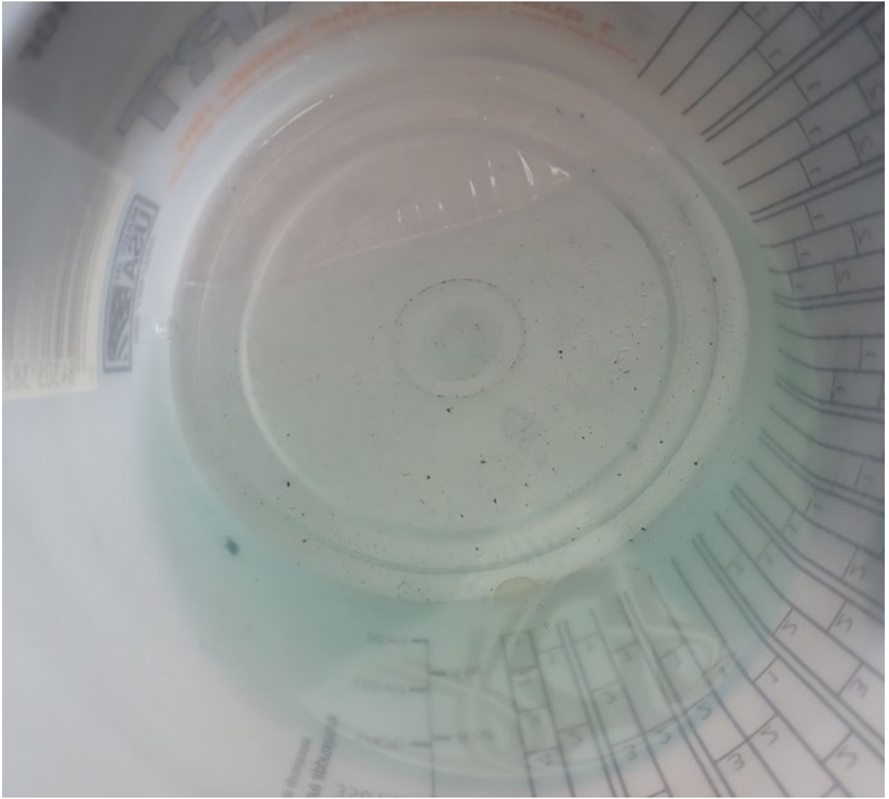
Figure 10 Fuel collected from the carburetor bowl.
