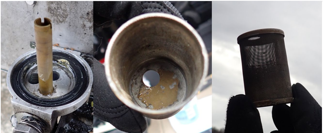
Figure 8 View of the gascolator mount and screen.
