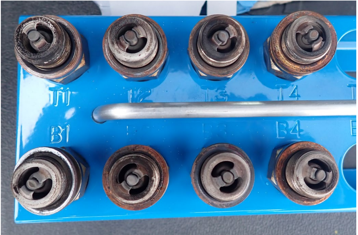
Figure 20 View of sparkplugs removed from the engine.
