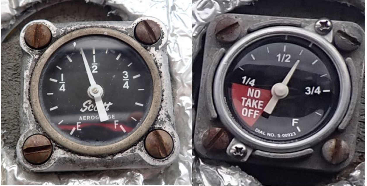
Figure 5 View of the left and right fuel level indicator from inside the cockpit.
