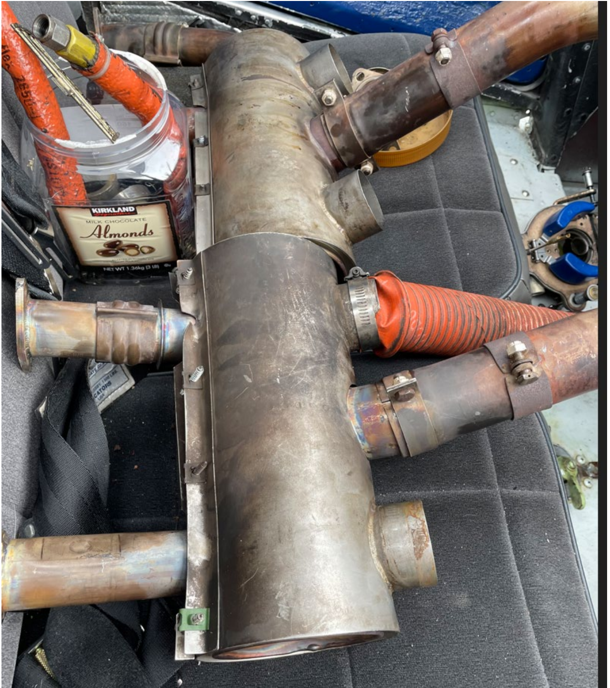
Figure 21 Left and right exhaust collectors and mufflers.
