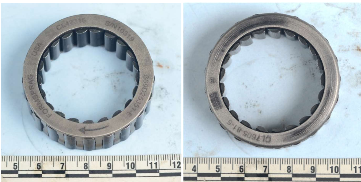
Figure 5 - Sprag Assembly, part number 369D25351-E (BSC)
