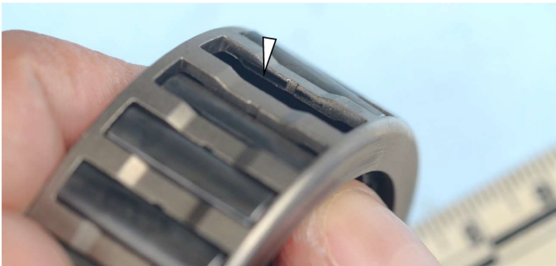
Figure 7 - Wear on sprag cage
