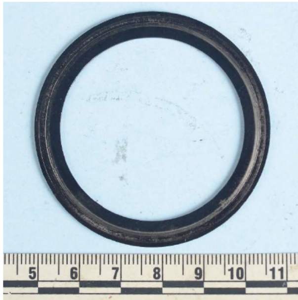
Figure 6 – Spacer/washer, part number 369A5360-BSC
