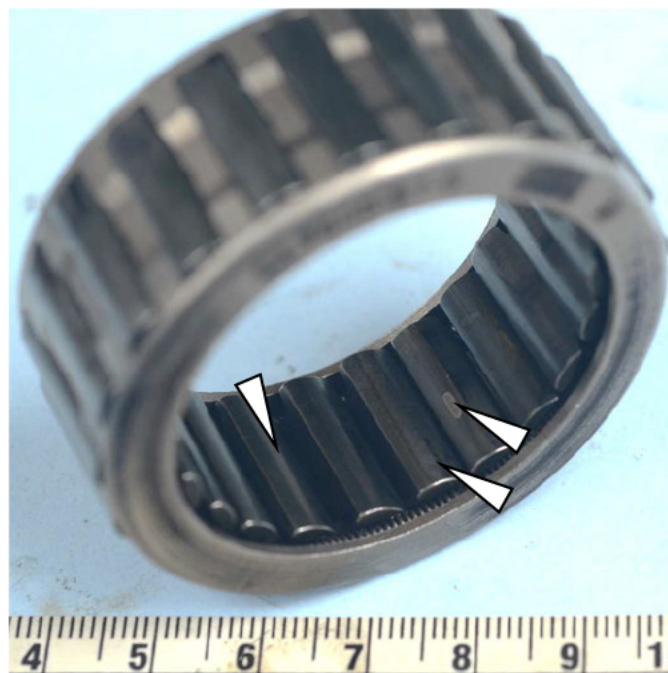
Figure 9 - Sprag assembly, showing flaking of the Formchrome surface treatment on one of the sprags, and wear on sprag load areas.
