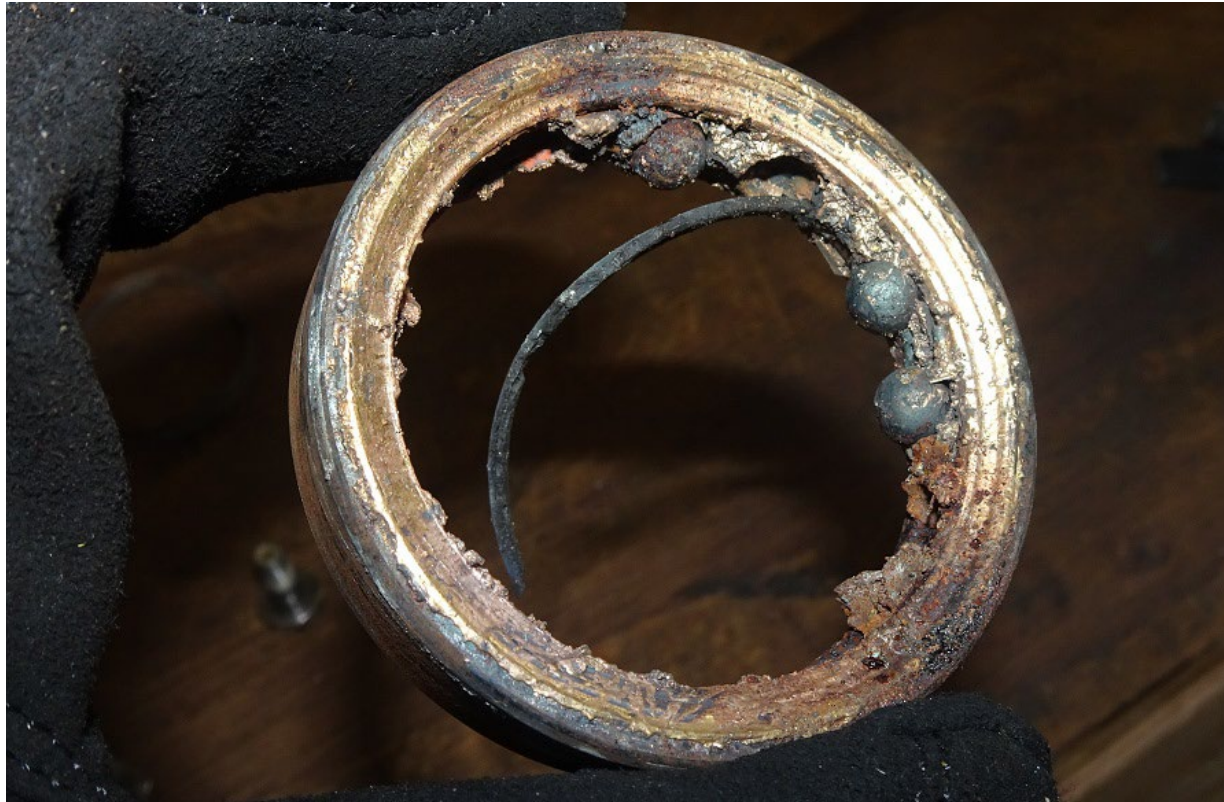
Photograph 3 - Image of clutch output bearing outer race with three roller elements adhered (NTSB Photo)
