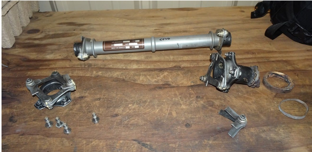
Photograph 2 - Image of Kaflex driveshaft after removal from wreckage (NTSB Photo)
