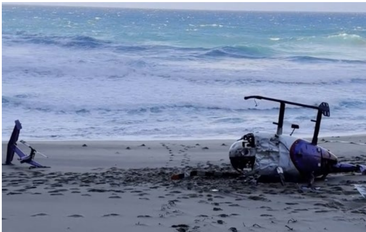
Photograph 1 - Image of fuselage and the separated empennage containing the vertical fin, horizontal stabilizer, and tail rotor (Courtesy of Operator)
