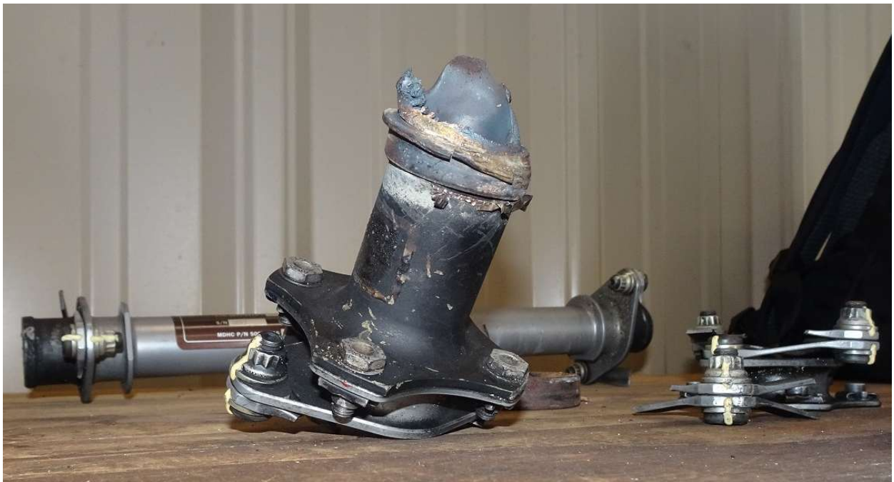
Figure 7. The forward portion of the clutch inner race still within the flanged connection attached to the aft flex plates of the Kaflex driveshaft.
