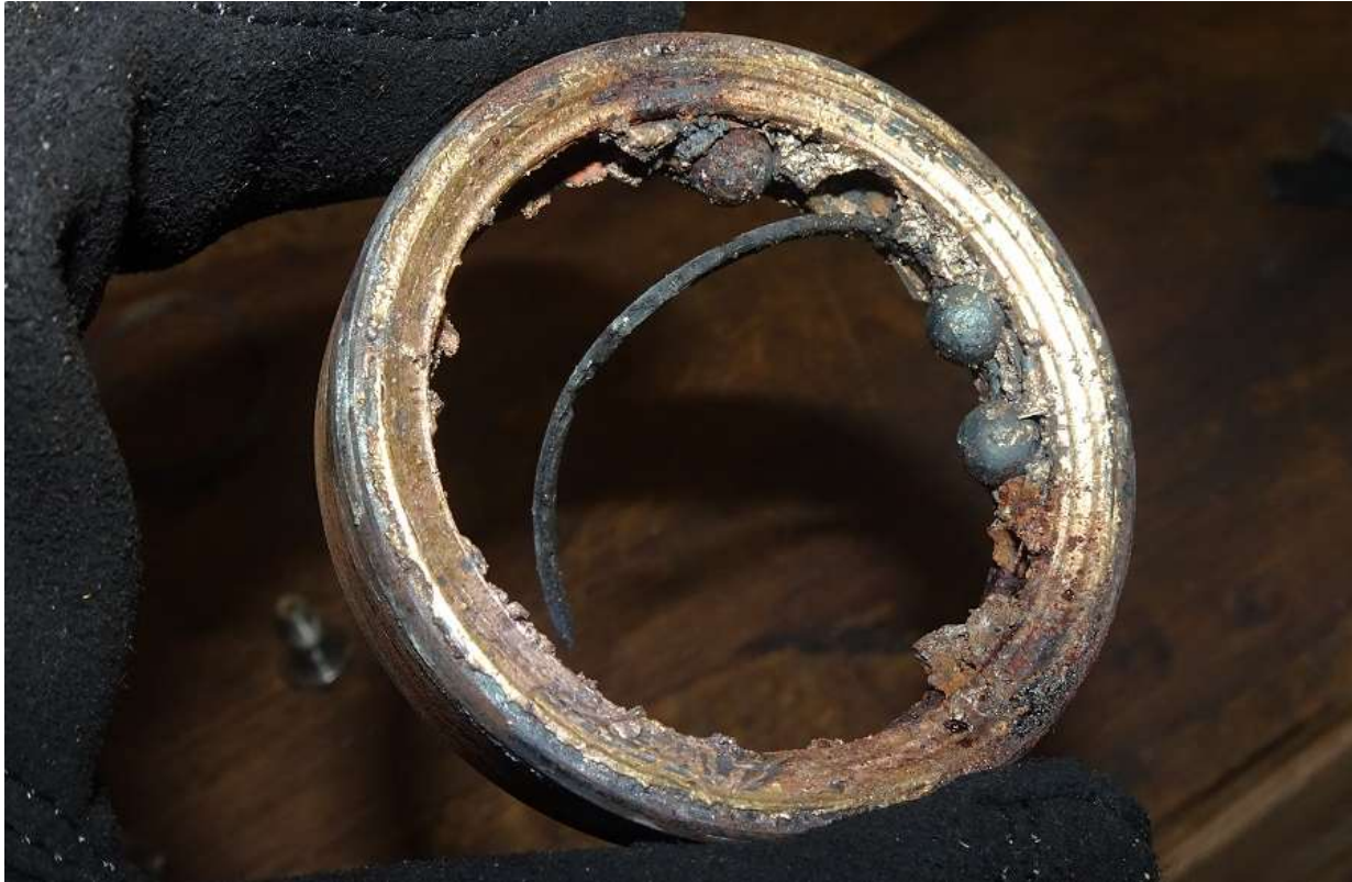
Figure 8. The clutch output bearing outer race with the three roller (ball) elements adhered.
