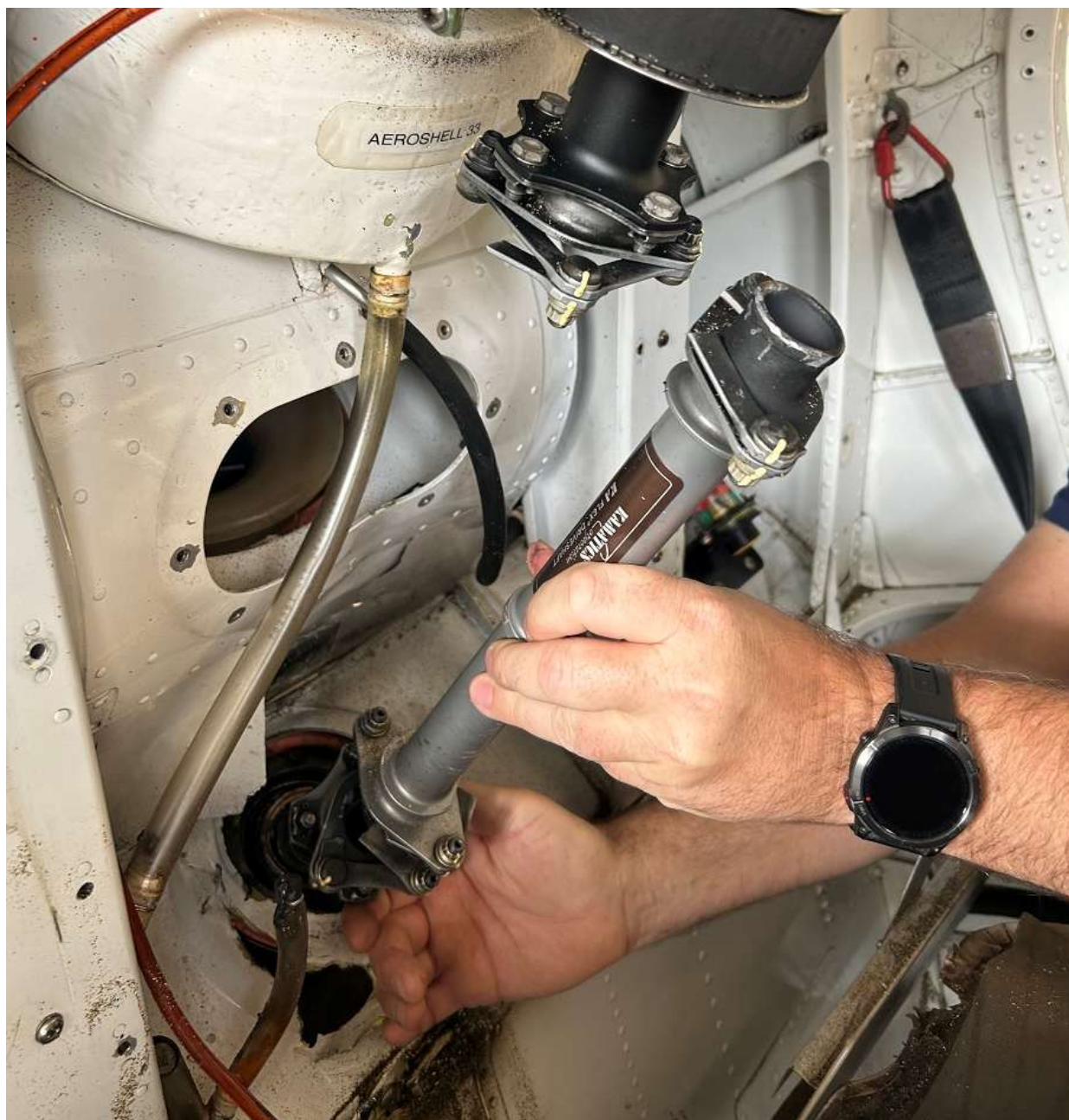
Figure 3. The Kaflex driveshaft as found in the wreckage after removal of the driveshaft cover. (Image courtesy of the FAA)
