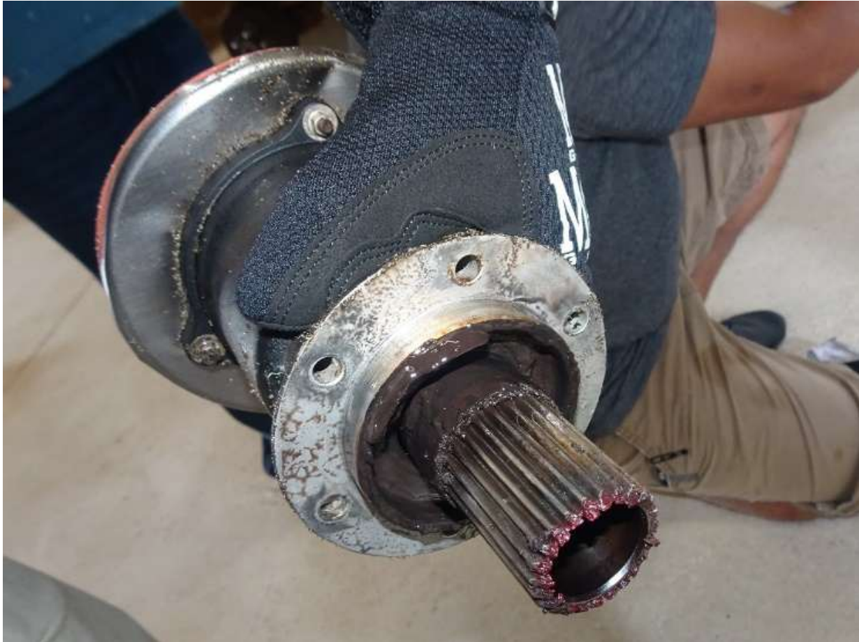
Figure 9. The clutch outer race splines after removal of the overrunning clutch assembly from the engine.
