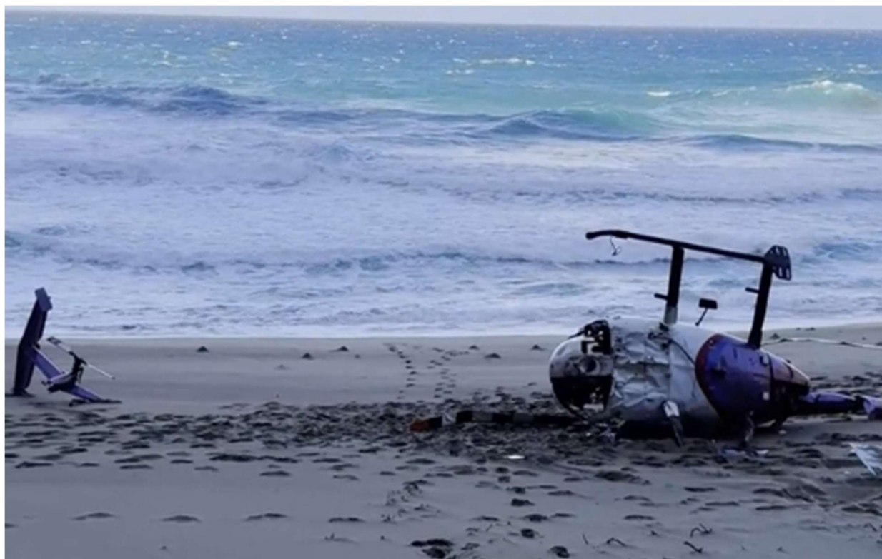
Figure 2. The main fuselage and the separated empennage containing the vertical fin, horizontal stabilizer, and tail rotor. (Image courtesy of Jack Harter Helicopter)
