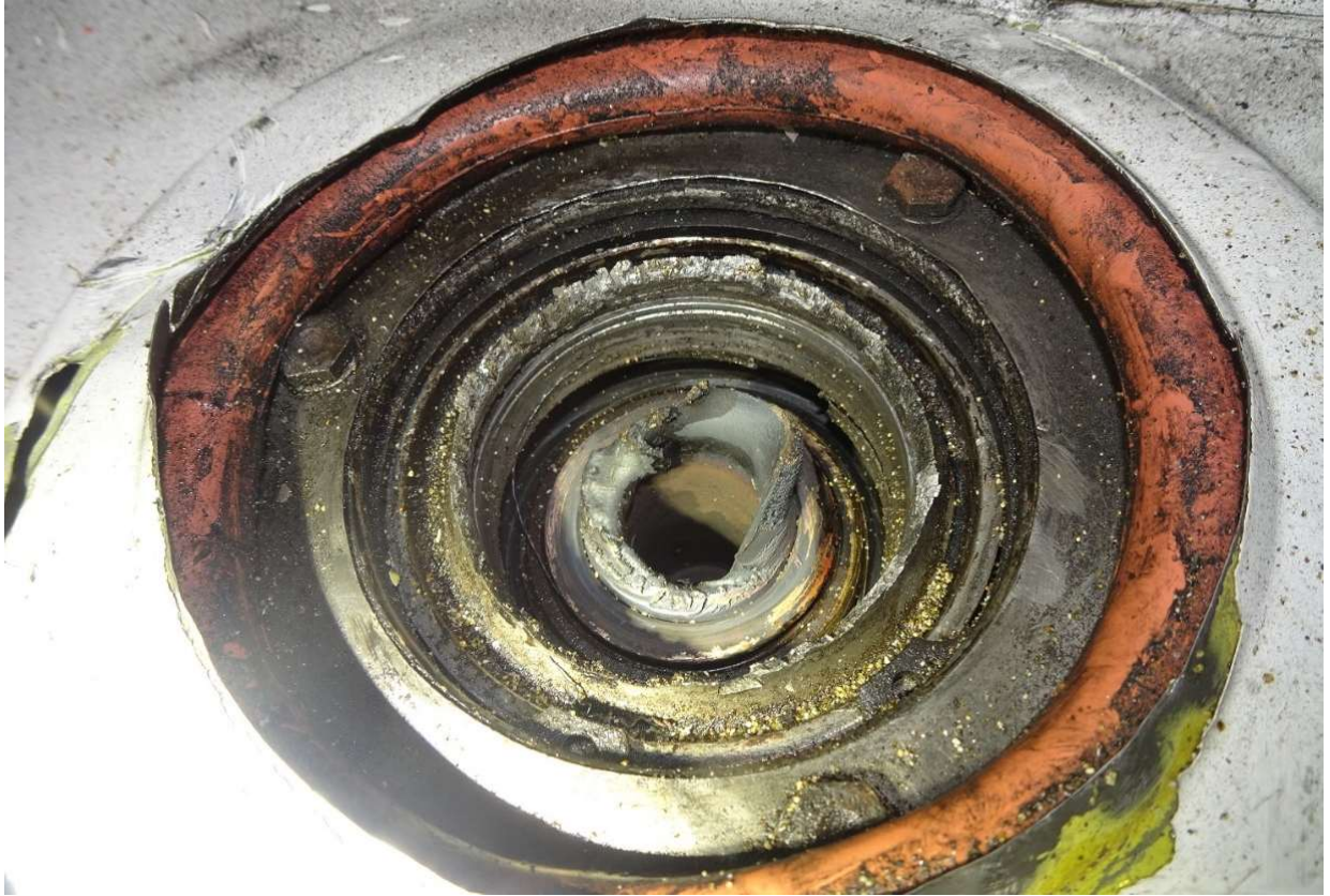
Figure 6. The fractured and thermally deformed clutch inner race.
