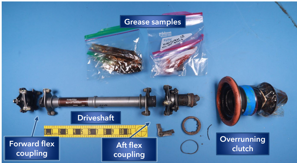
Figure 1. Overall view of the submitted components and grease samples.
