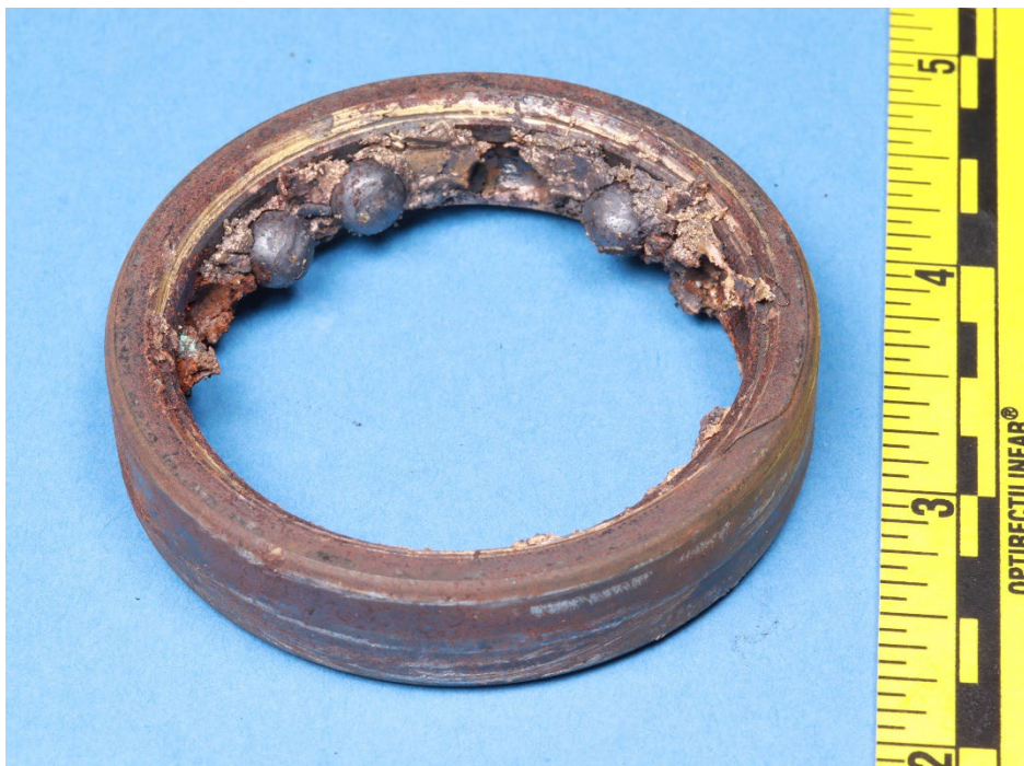
Figure 4. Output bearing outer race with cage and ball remnants.
