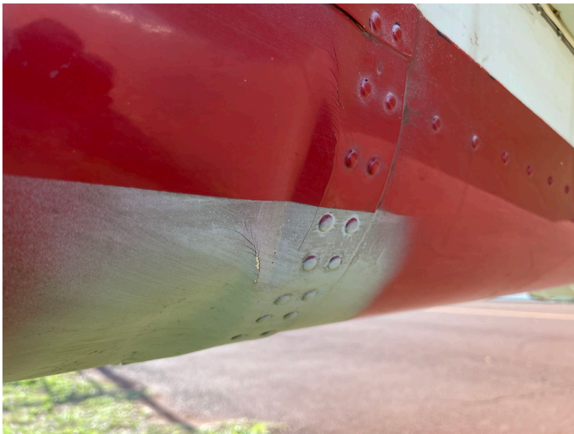
Photograph 2 -Image of damage to the fuselage (Courtesy of FAA)
