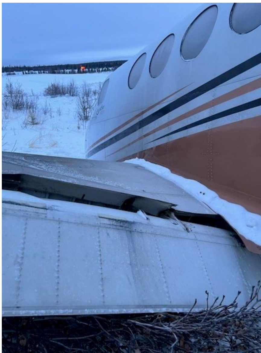
Photograph 2 - Image of the left wing root section viewed from the rear (Courtesy of Operator)
