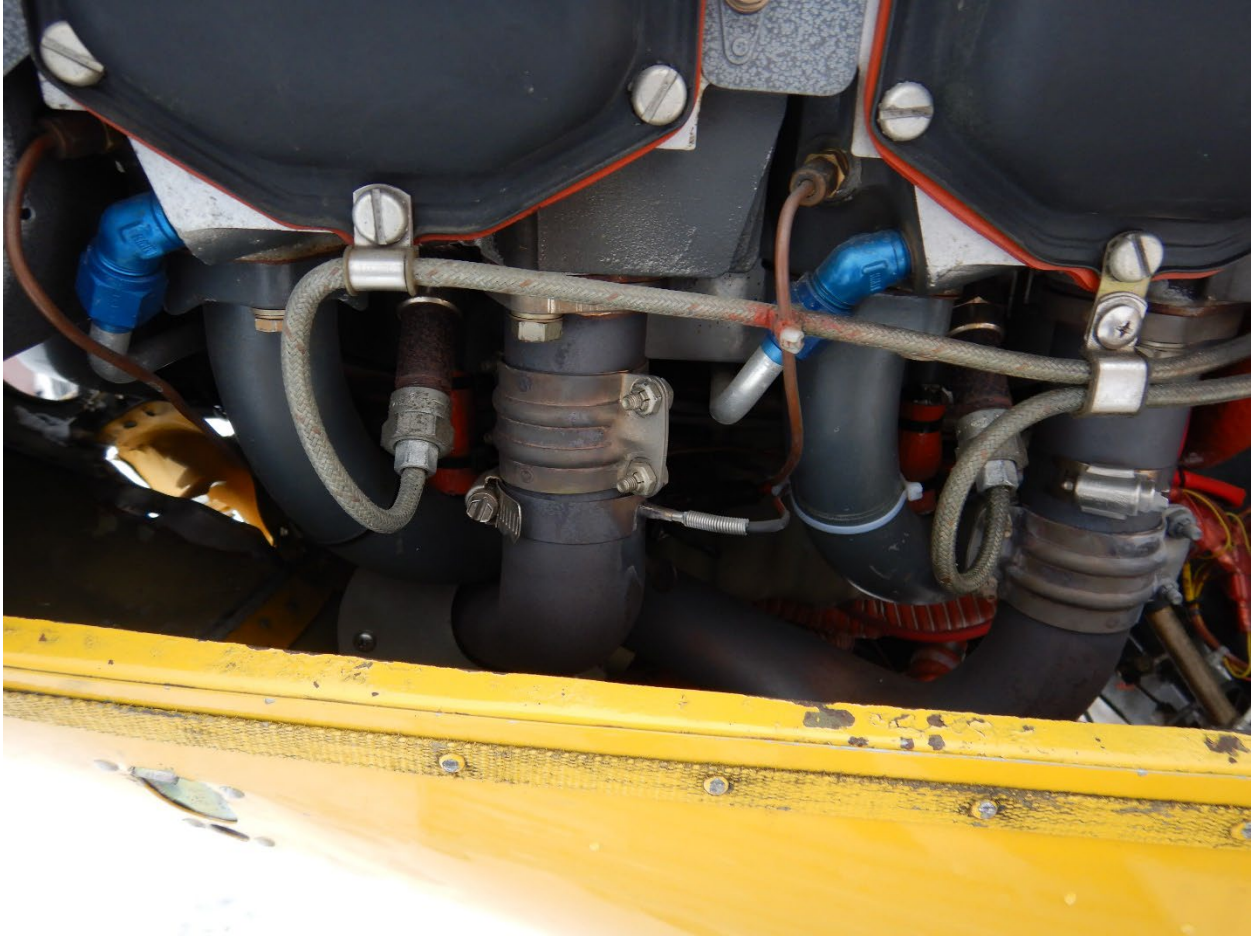
Figure 10 Left side view the engine exhaust collectors and air intake.
