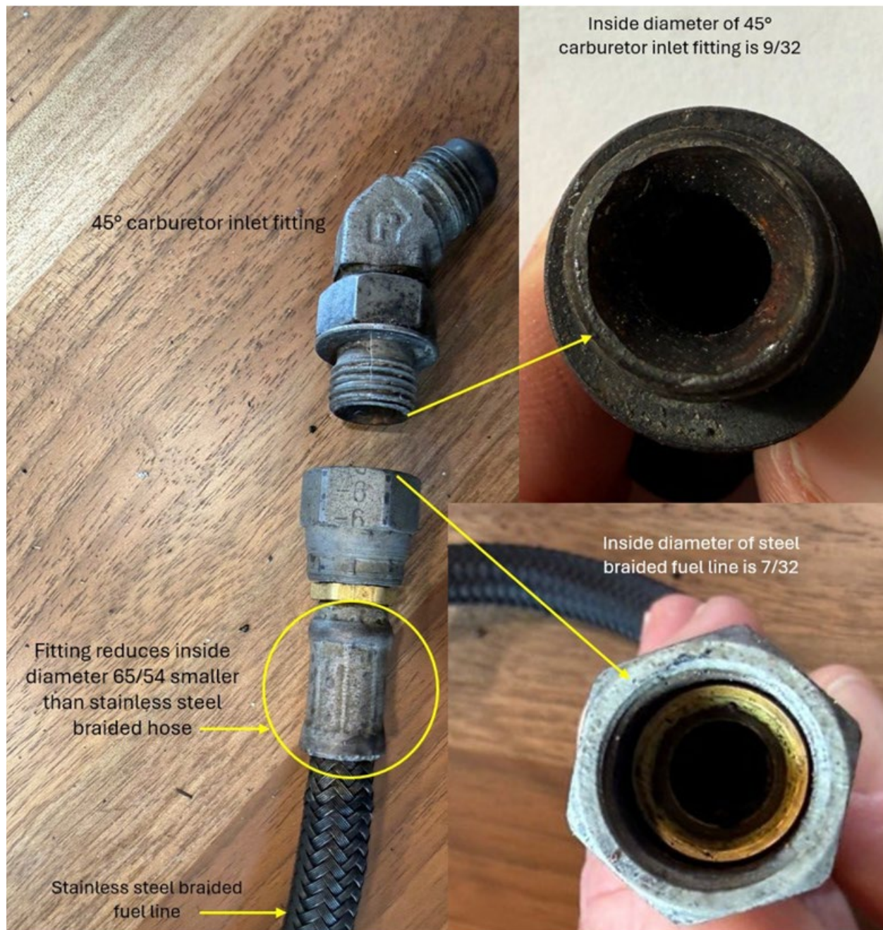
Figure 8 Inside diameter of inlet fitting and steel braided line
