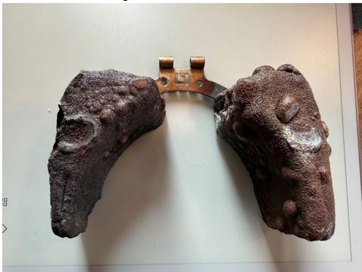
Figure 15 Foam floats from inside the carburetor
