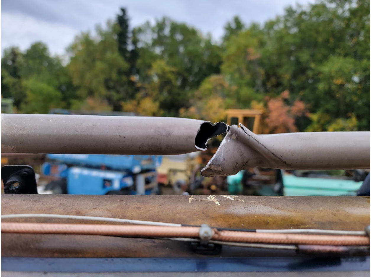
Figure 12 View of torsional damage to the tail rotor driveshaft.
