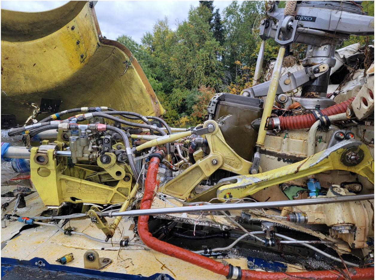
Figure 16 View of the left side of the hydraulic servos and main transmission.
