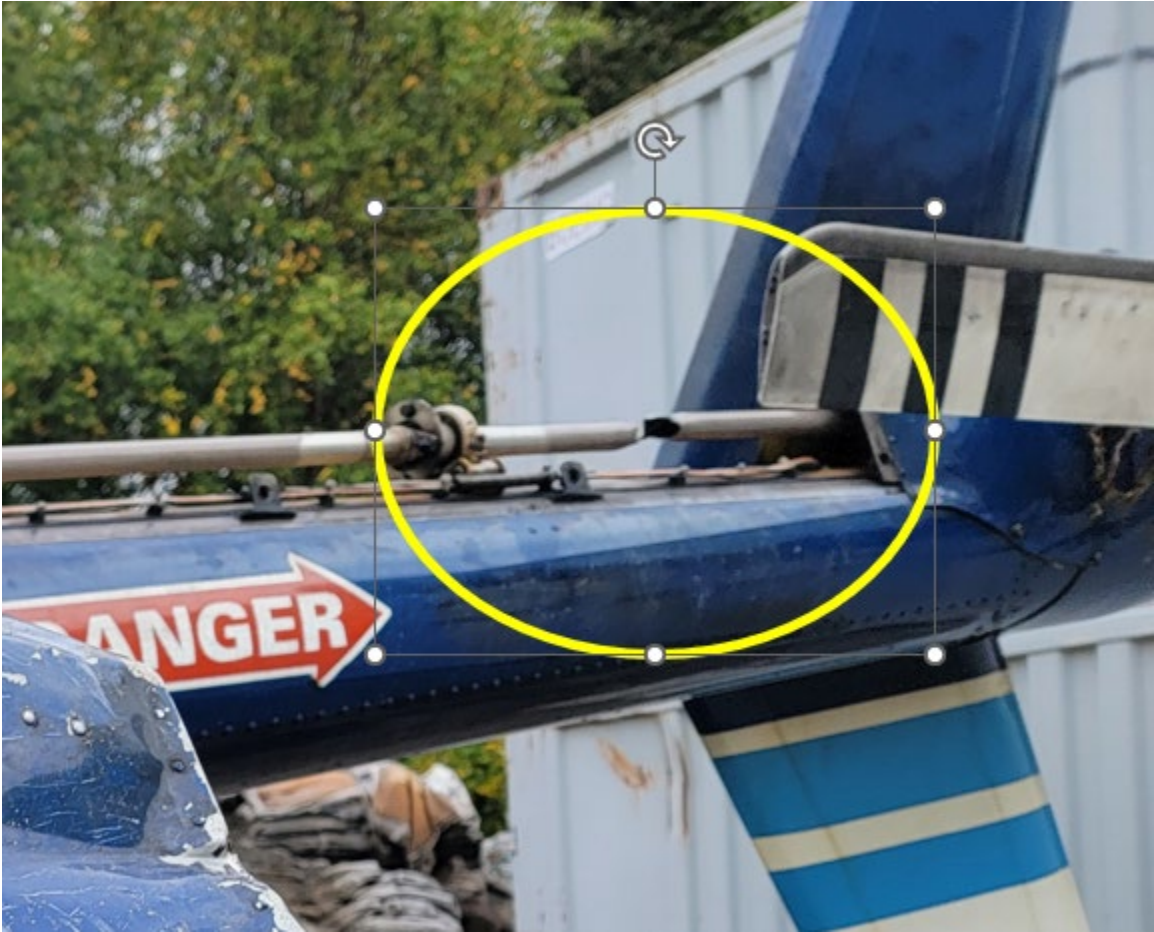
Figure 11 view of the location of the torsional damage to the tail rotor driveshaft.
