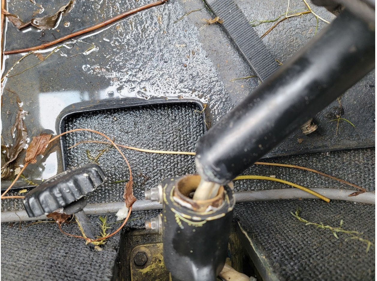
Figure 17 View of the cyclic control fracture.
