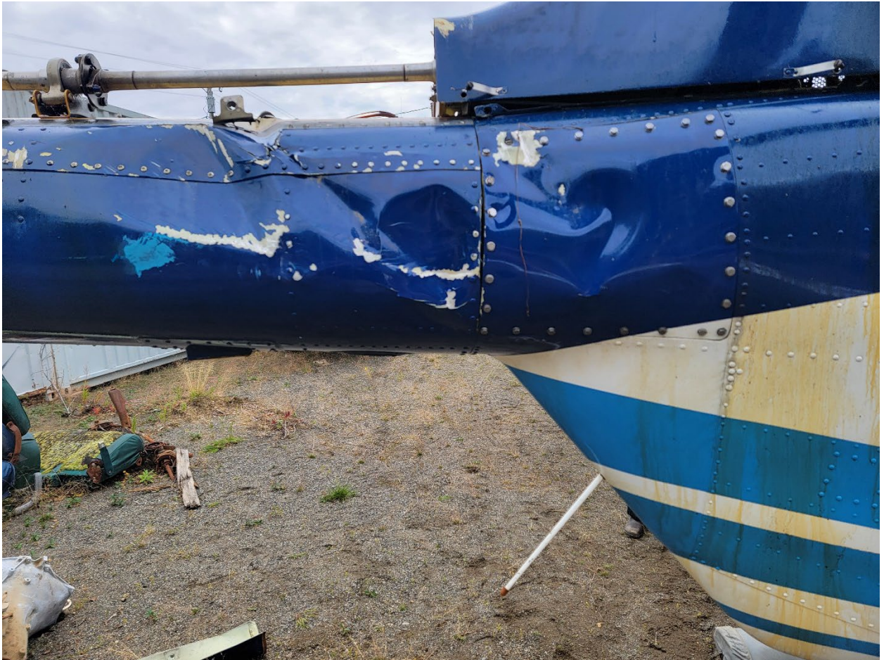
Figure 6 view of the tail boom attachment to the fuselage.
