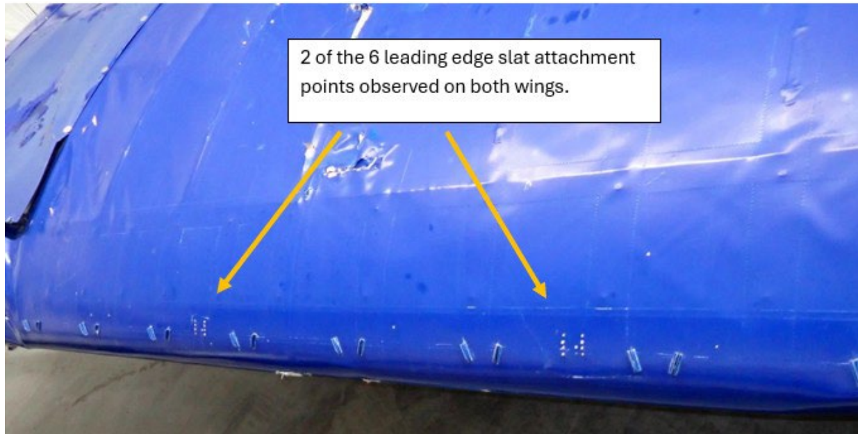
Figure 11 Leading edge slat attachment points
