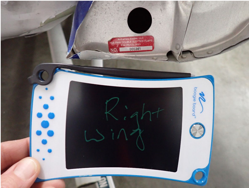
Figure 10 Right wing PSTOL flap data tag
