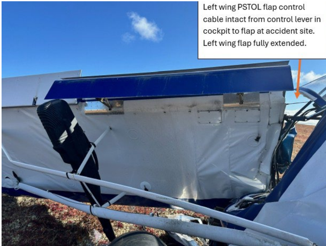
Figure 6 Left wing PSTOL flap with cable attached
