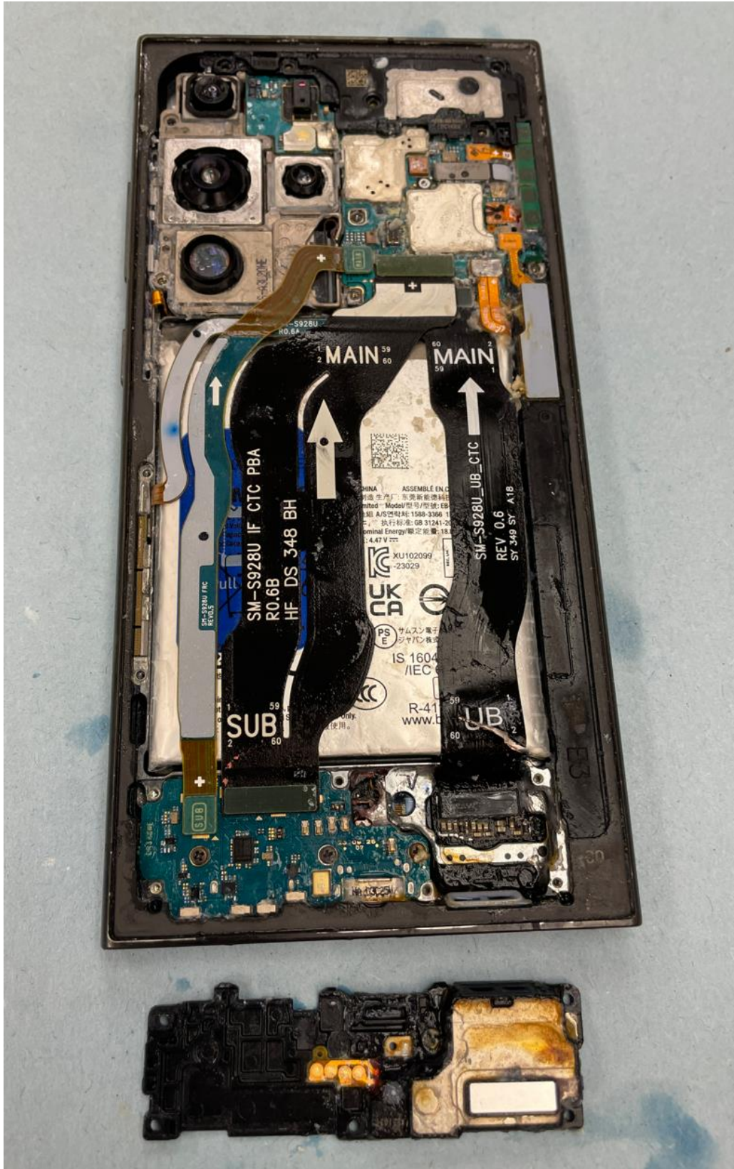
Figure 3. The interior of the Samsung phone showed severe water damage.
