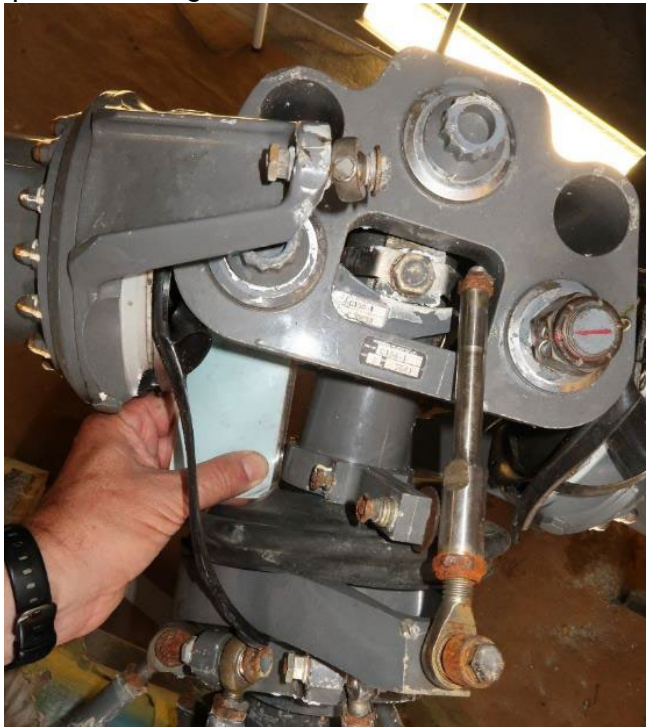
Figure 8 Rotor head and mast illustrating the bend of the drive shaft and the broken pitch link.
