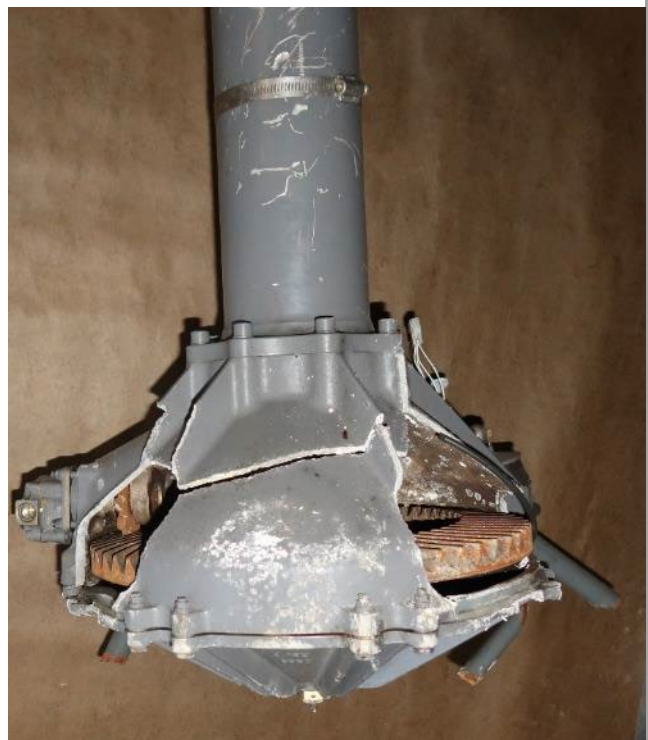
Figure 7 Foreword end of the gear box with case separations, and revealing the ring gear.
