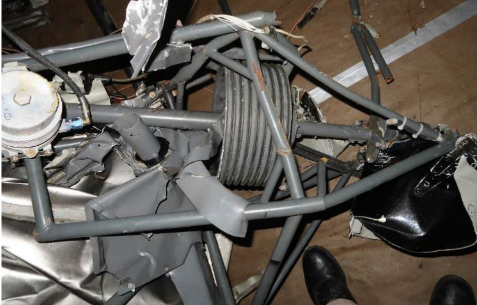
Figure 3 Aft airframe structural members showing right to left deformation.
