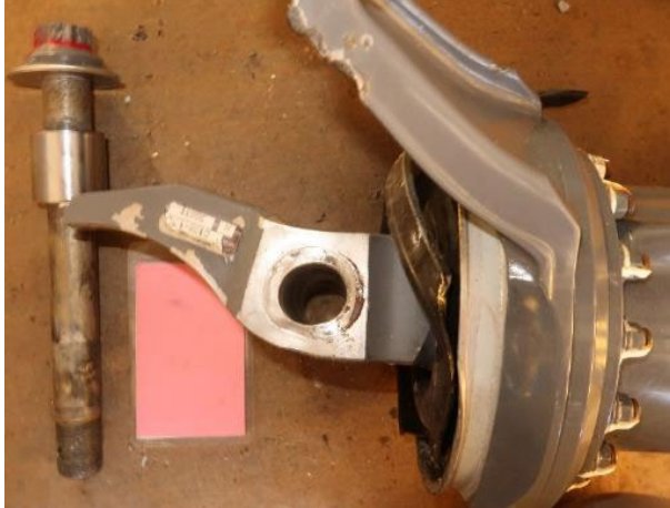
Figure 14 Pitch bolt and spindle tusk.
