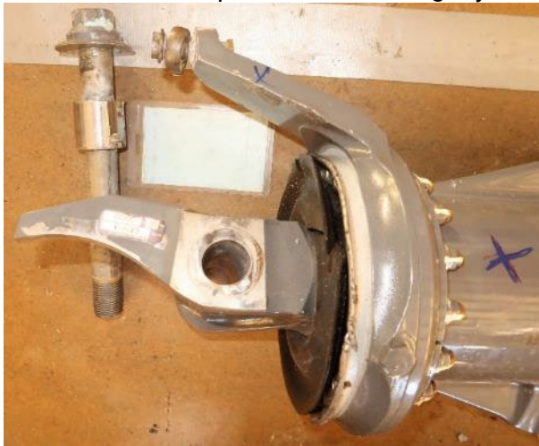
Figure 12 Pitch bolt and spindle tusk.
