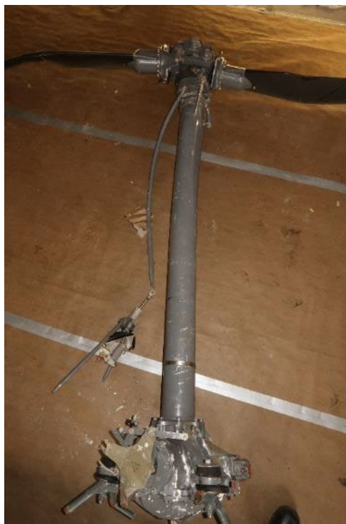
Figure 6 Main rotor gearbox, mast, and rotor head.
