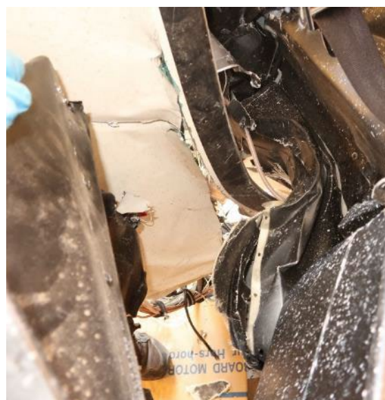
Figure 5 Crushed cabin floor structure deformed semi circularly aligned with the leading edge of the main rotor blade.
