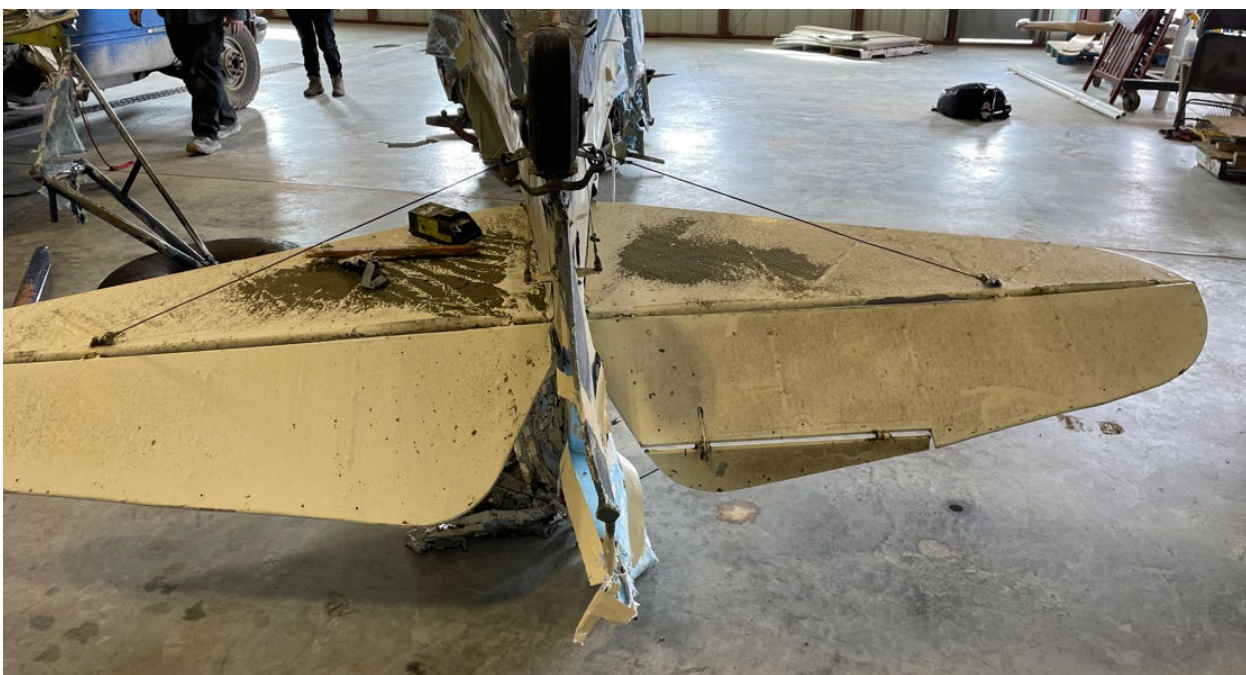
Figure 9 The underside view of the left and right horizontal stabilizers and elevators.
