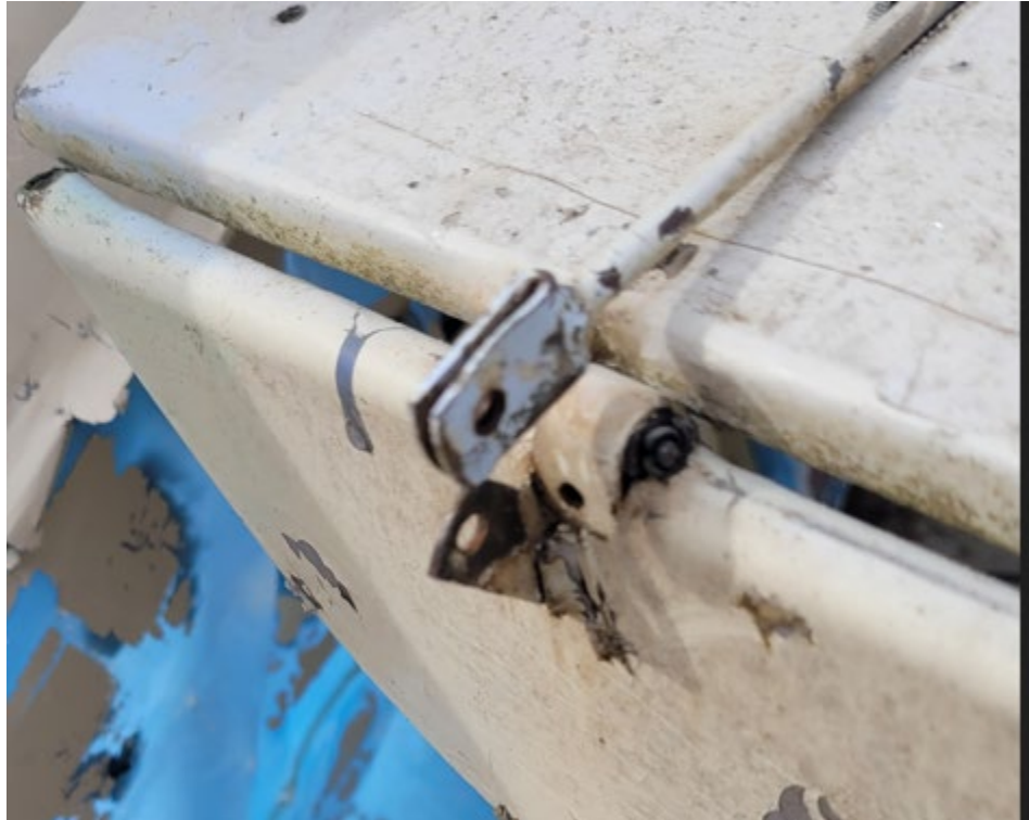
Figure 10 view of missing bolt in the attachment of the control cable to the elevator trim tab.
