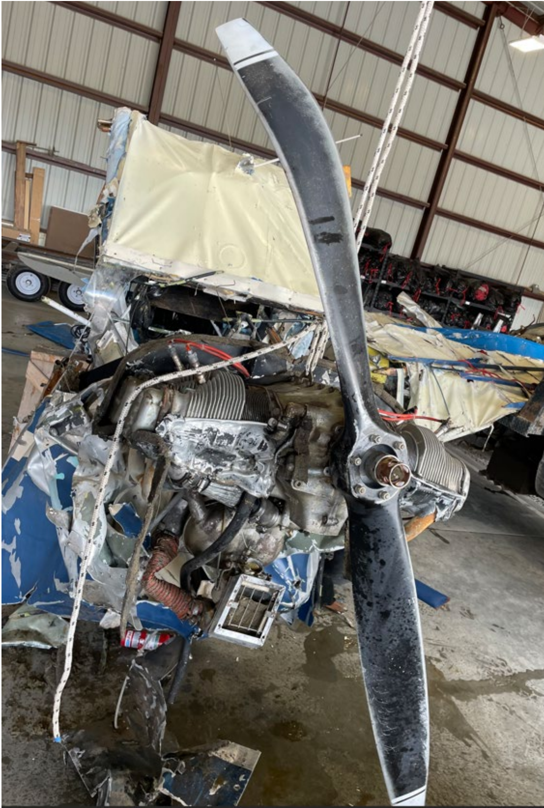
Figure 20 View of impact damage to the front of the engine and damage to the engine propeller.
