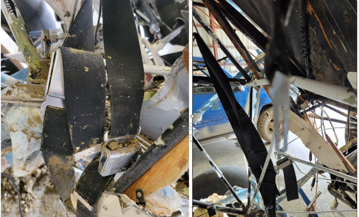
Figure 14 View of buckles and unattached shoulder harness.
