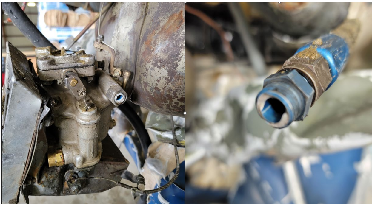
Figure 15 View of fuel line connection into the carburetor.
