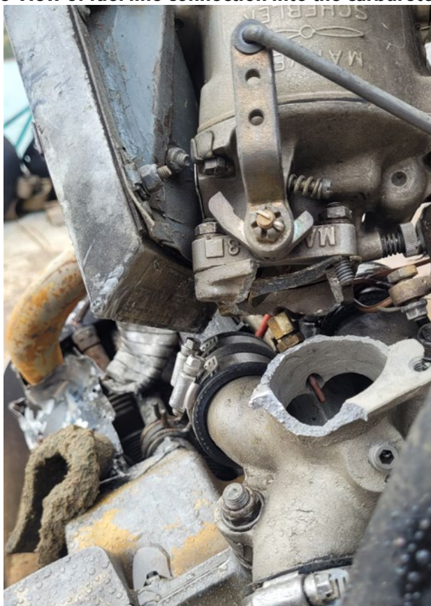
Figure 16 View of facture break between the carburetor and induction system.
