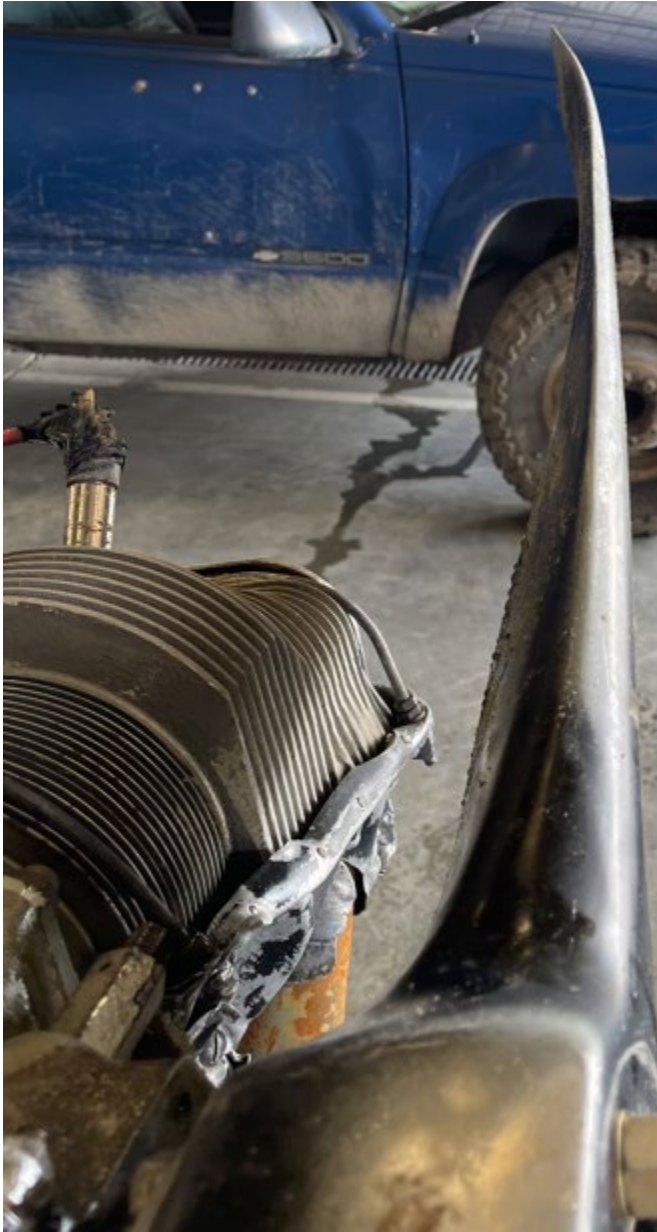
Figure 26 View of damage to the other side of the propeller.
