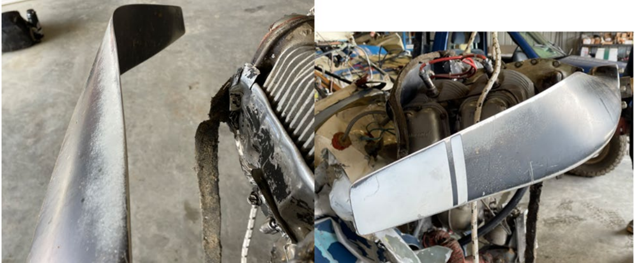
Figure 25 View of the damage to one side of the propeller.
