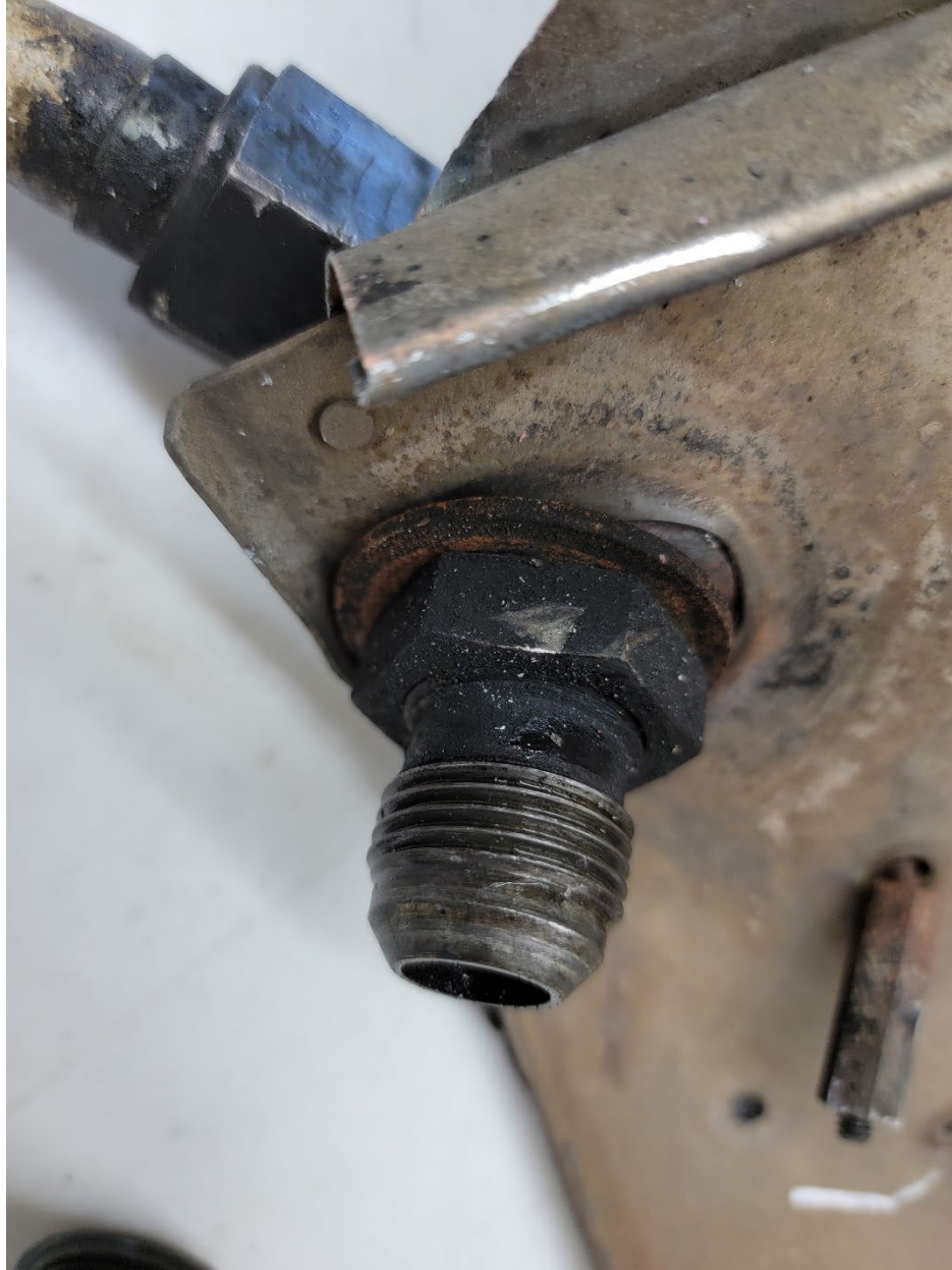
Figure 4. View of the undamaged fitting connected to the firewall.
