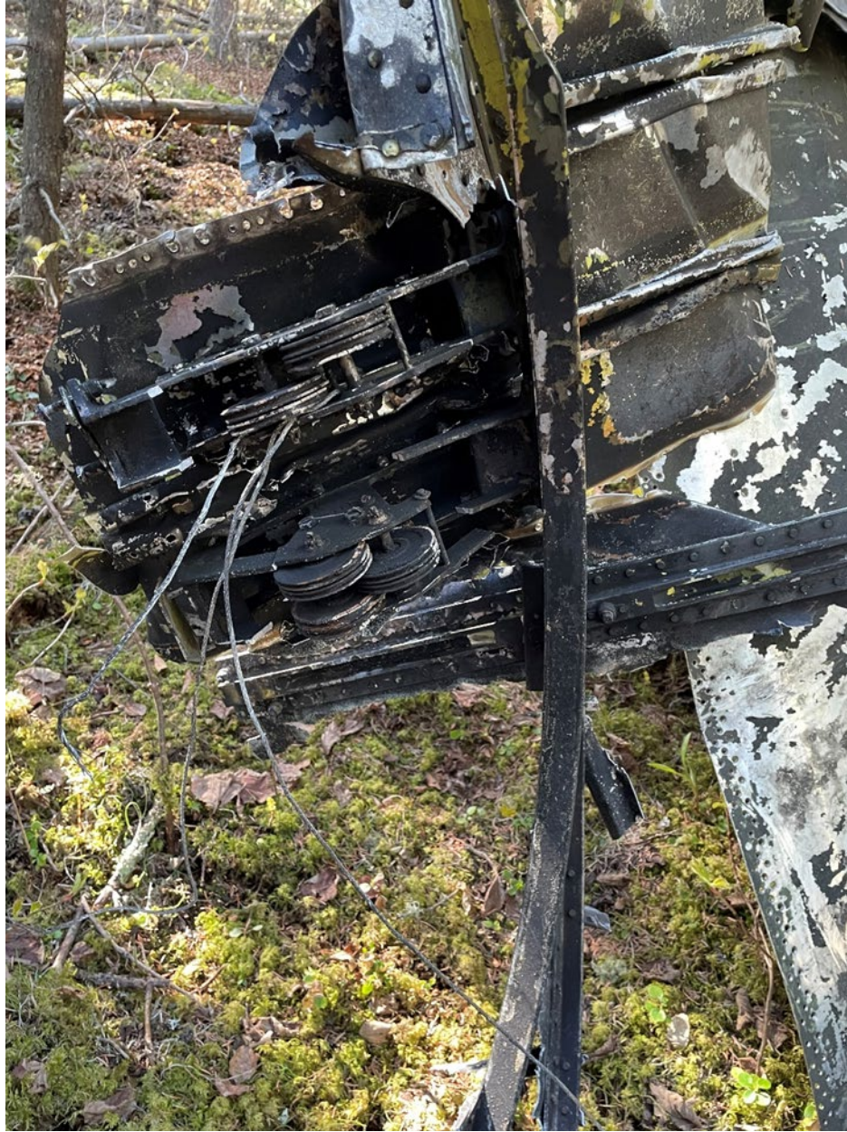
Figure 10 View of the left wing aileron control bell housing.
