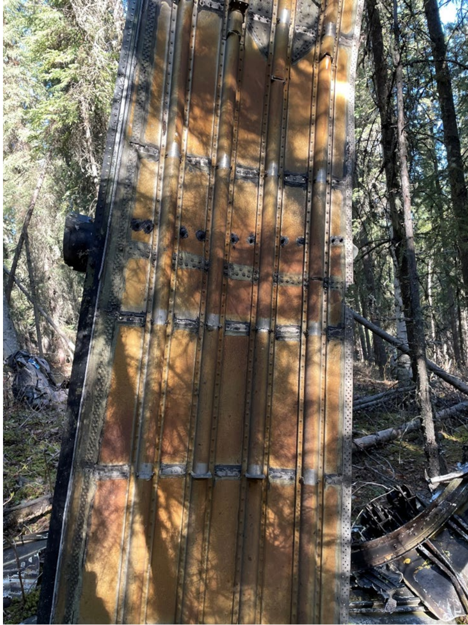
Figure 9 View of the underside of the large section of the upper left wing.
