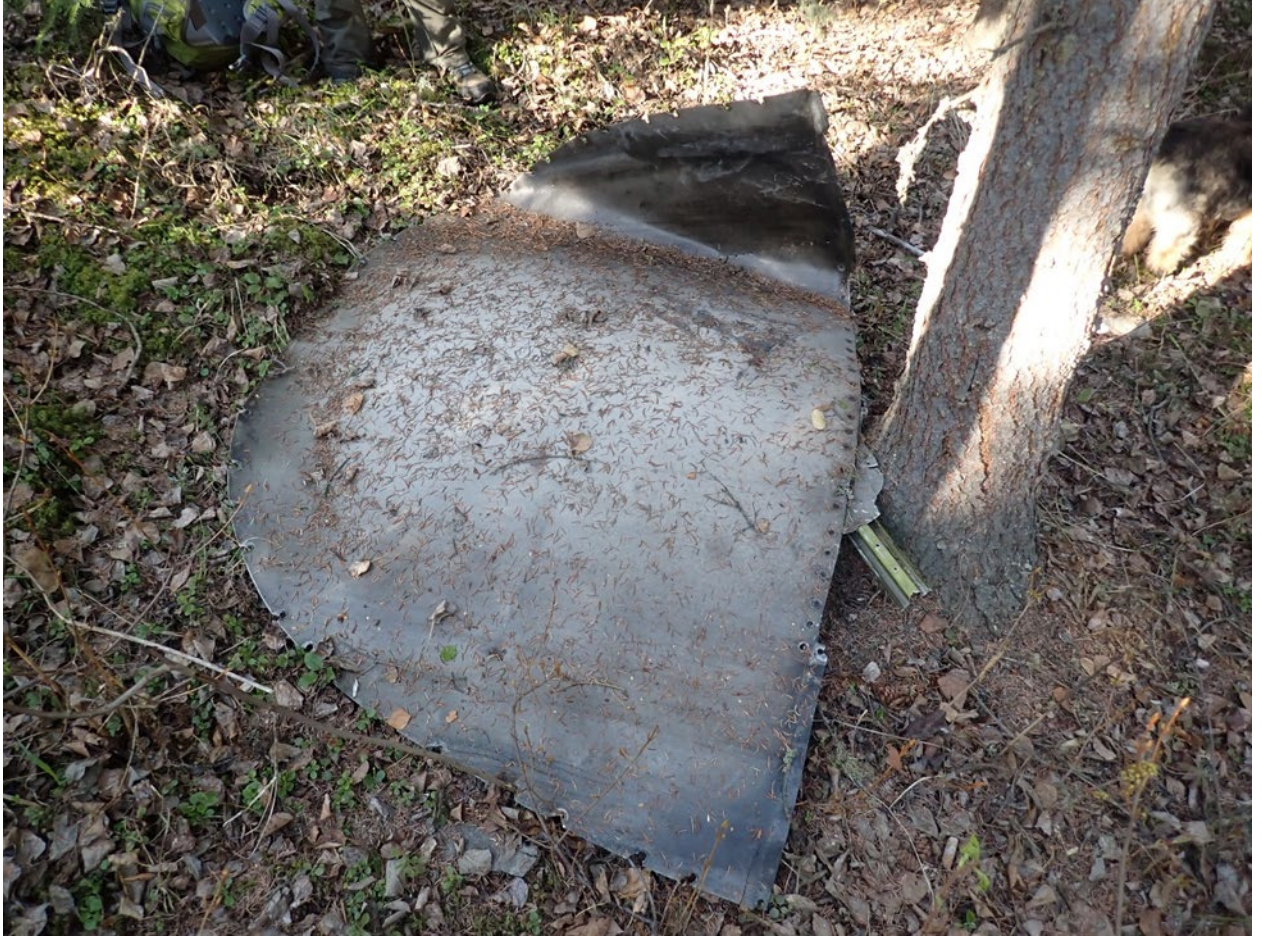
Figure 12 Section of the upper portion of the left wing.
