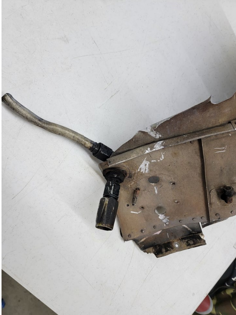
Figure 3. View of the AN-8 nut connected to the firewall fitting. Matching up the two parts found in the wreckage.
