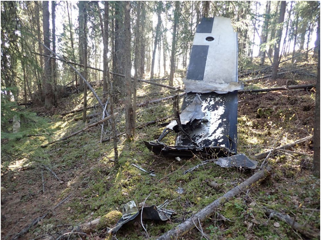
Figure 8 View of the top side of the upper left wing.
