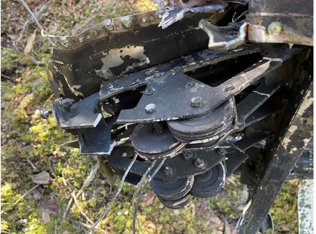
Figure 11 View of the left wing aileron control bell housing.
