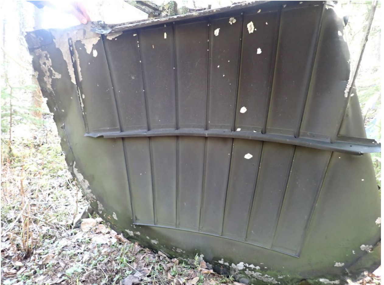
Figure 13 View of the underside of the upper section of the left wing.
