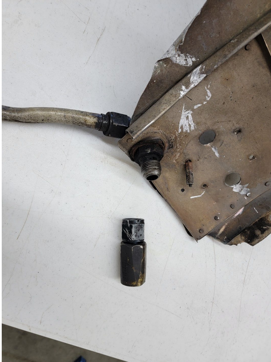
Figure 2 Firewall connection of the propeller feathering system.
