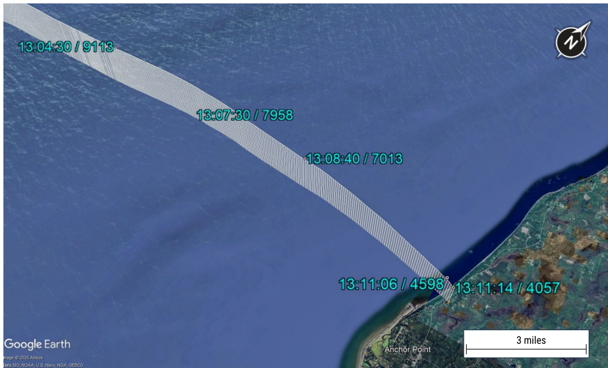
Figure 4. GPS flight path with selected times and altitudes notated.
