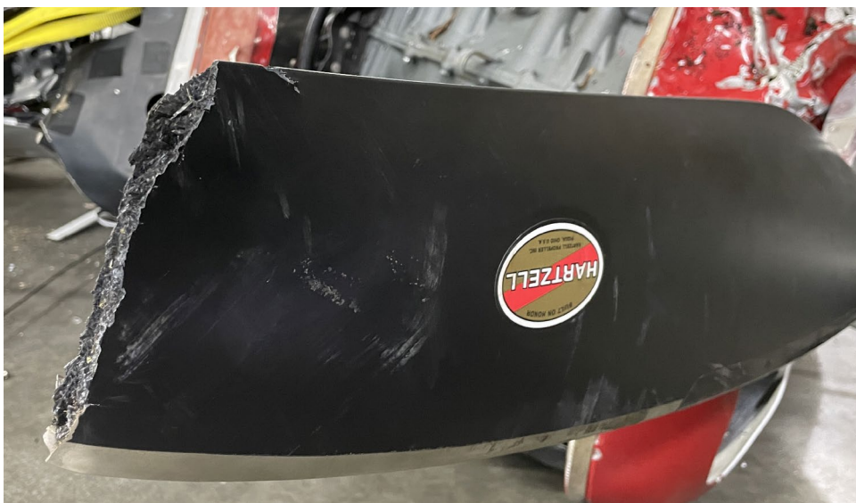
Figure 11. Propeller blade with missing tip, camber side (NTSB photo)
