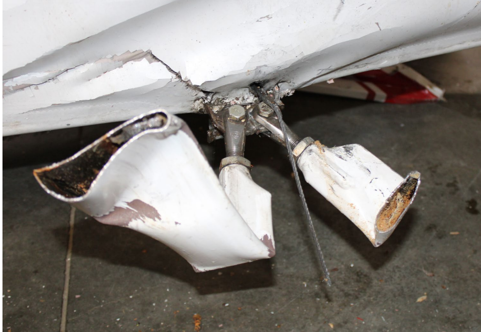
Figure 7. Left lift struts, lower ends, attached to fuselage (NTSB Photo)
