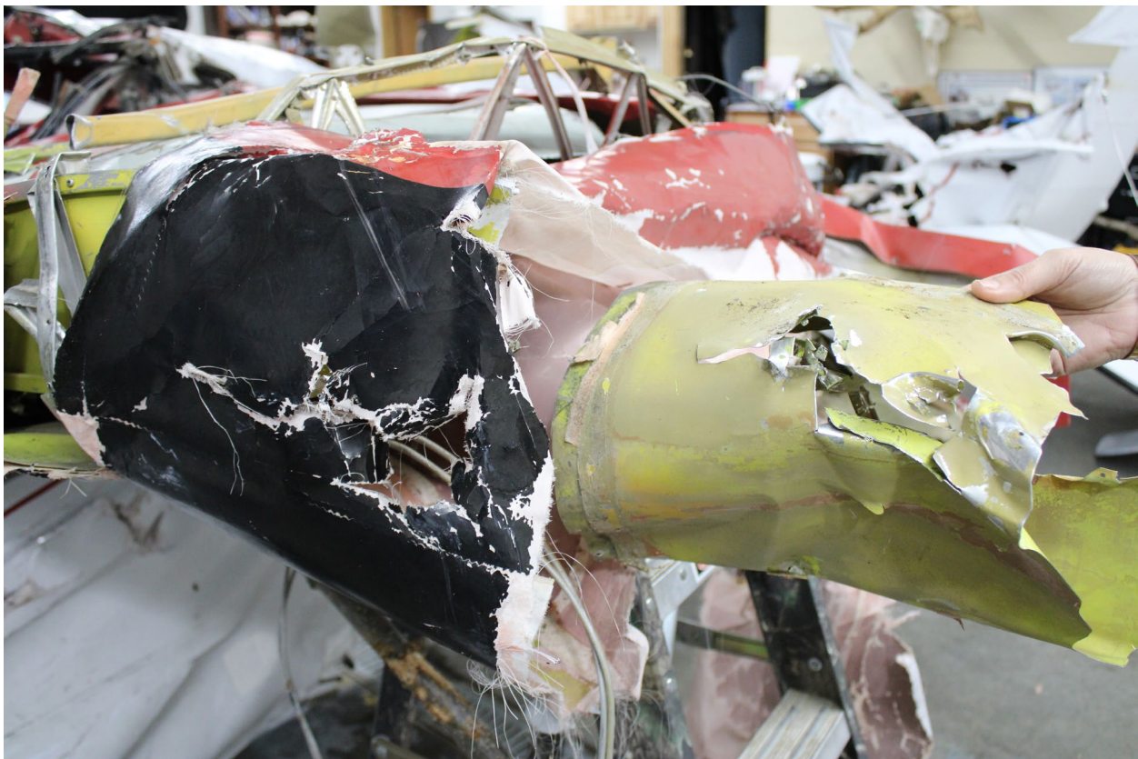
Figure 5. Left wing leading edge skin and fabric damage (NTSB photo)
