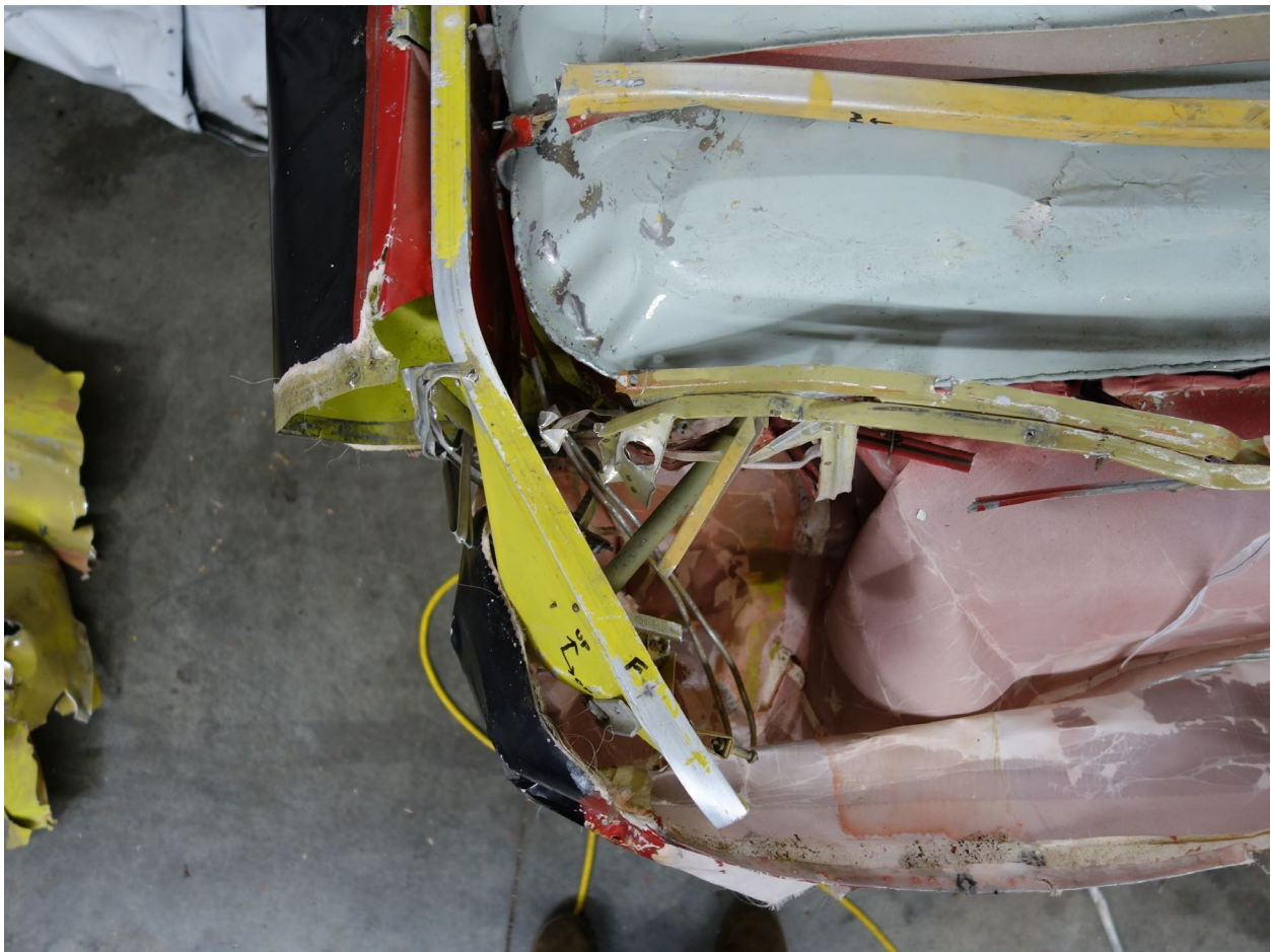
Figure 3. Left wing forward spar fracture, looking down (Piper photo)
