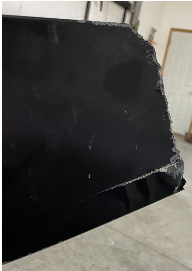
Figure 12. Propeller blade with missing tip, face side (NTSB photo)
