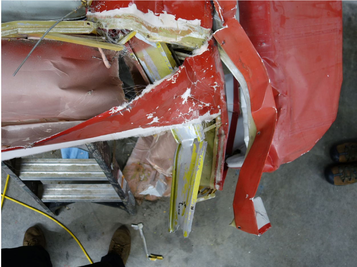
Figure 4. Left wing aft spar fracture, looking down (Piper photo)
