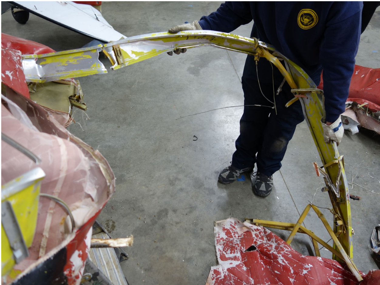
Figure 6. Left wing aft spar deformation (NTSB Photo)
