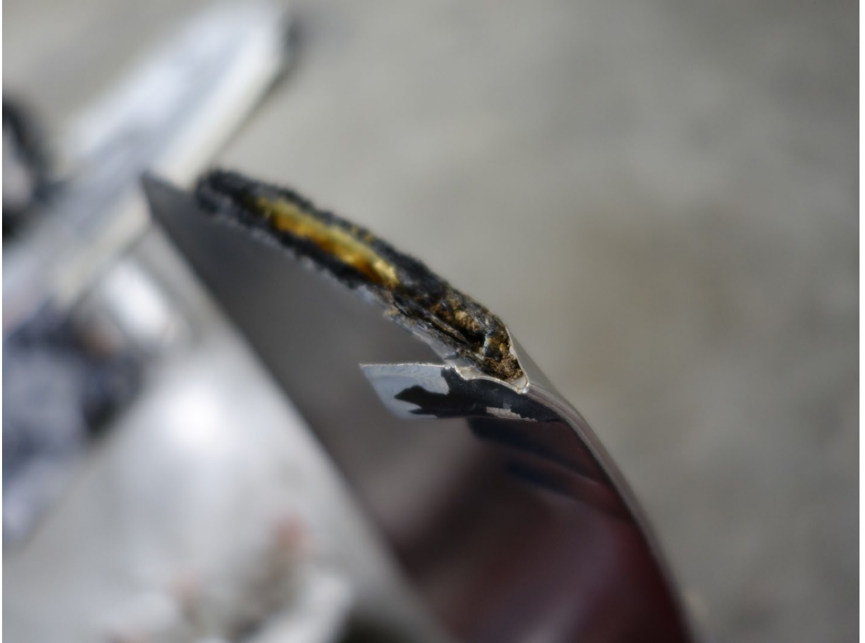
Figure 17 No.2 propeller blade separation point
