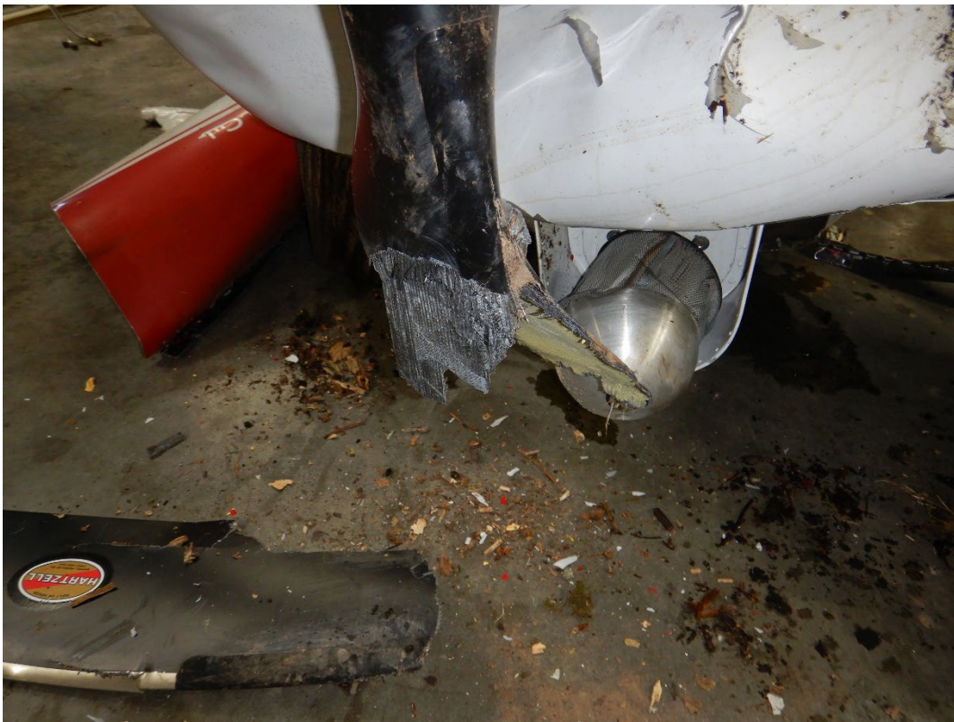
Figure 13 No.1 propeller blade view of separation point
