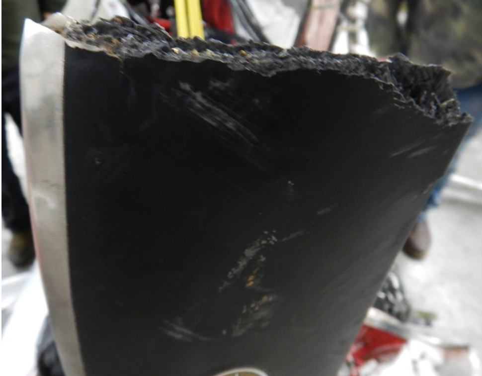
Figure 15 No.2 propeller blade separation point
