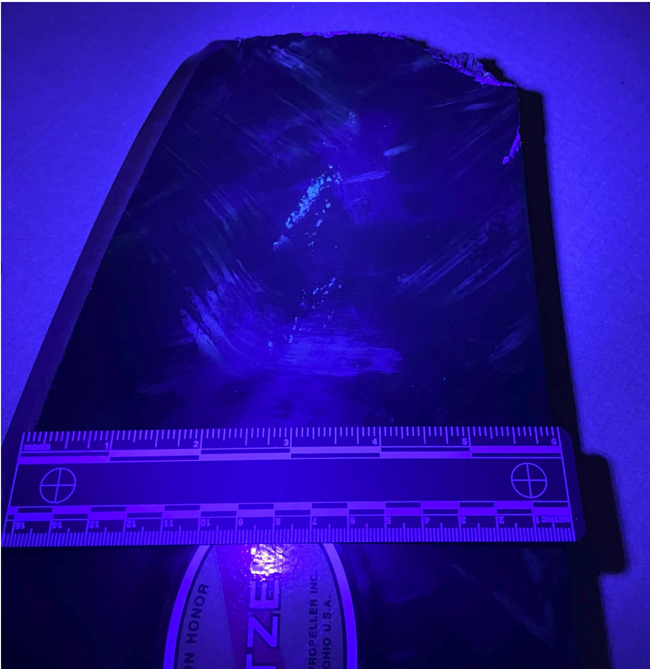
Photograph of front surface of blade under UV light
