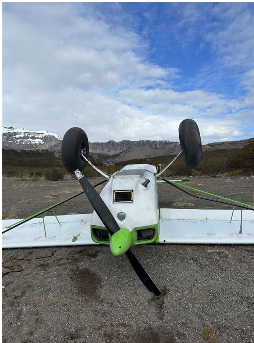
Photograph 2 - View of nose and bent wing strut (Courtesy of Pilot)
