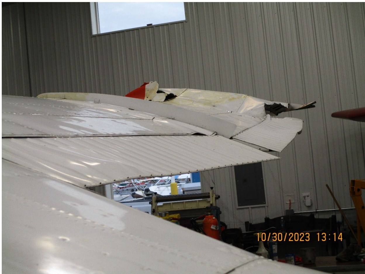
Figure 1 View of damage to right wing. (Courtesy of FAA)
