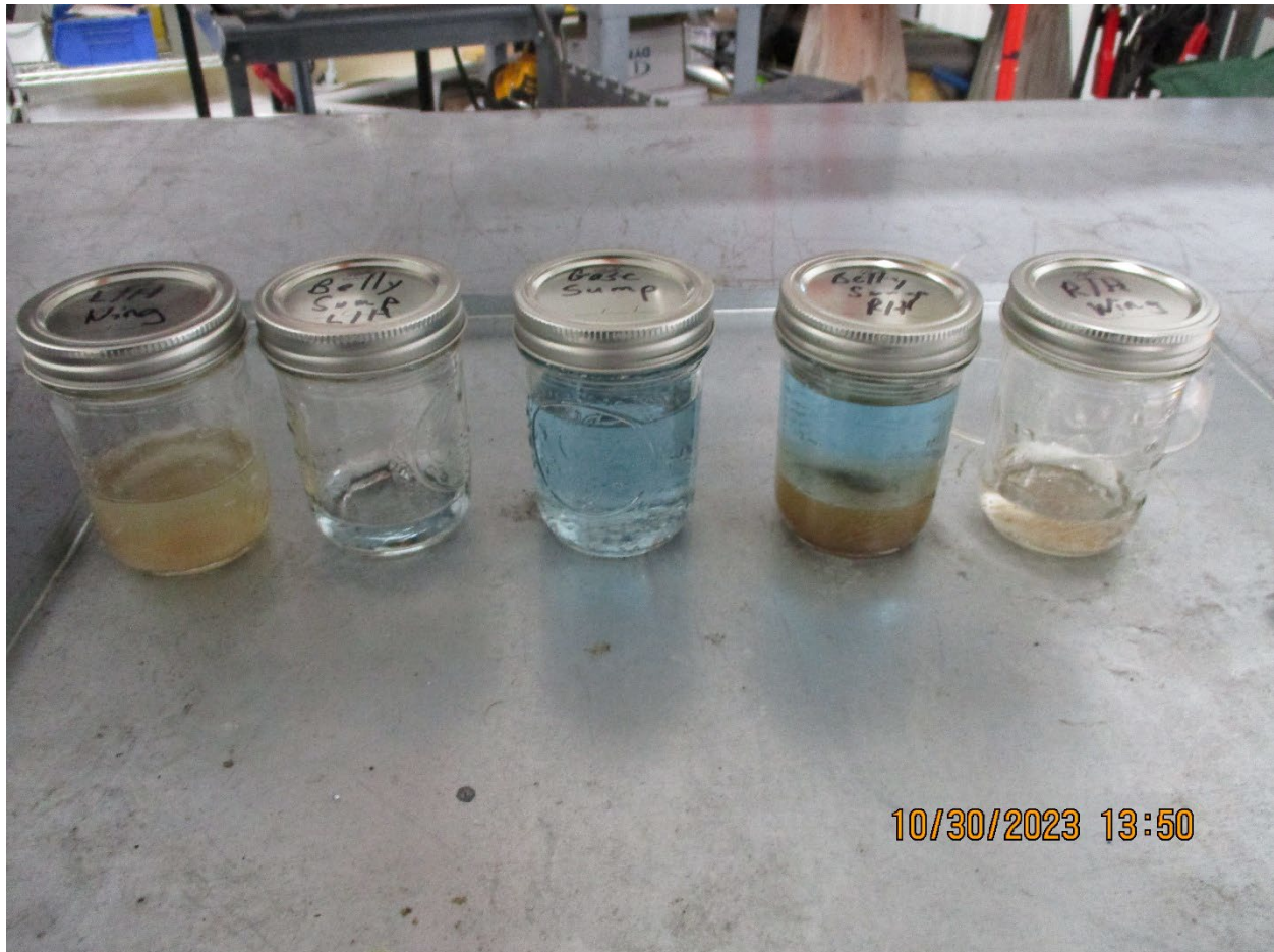
Figure 4 Fuel samples from the left wing, left belly sump, gascolator, right belly sump, and right wing.
