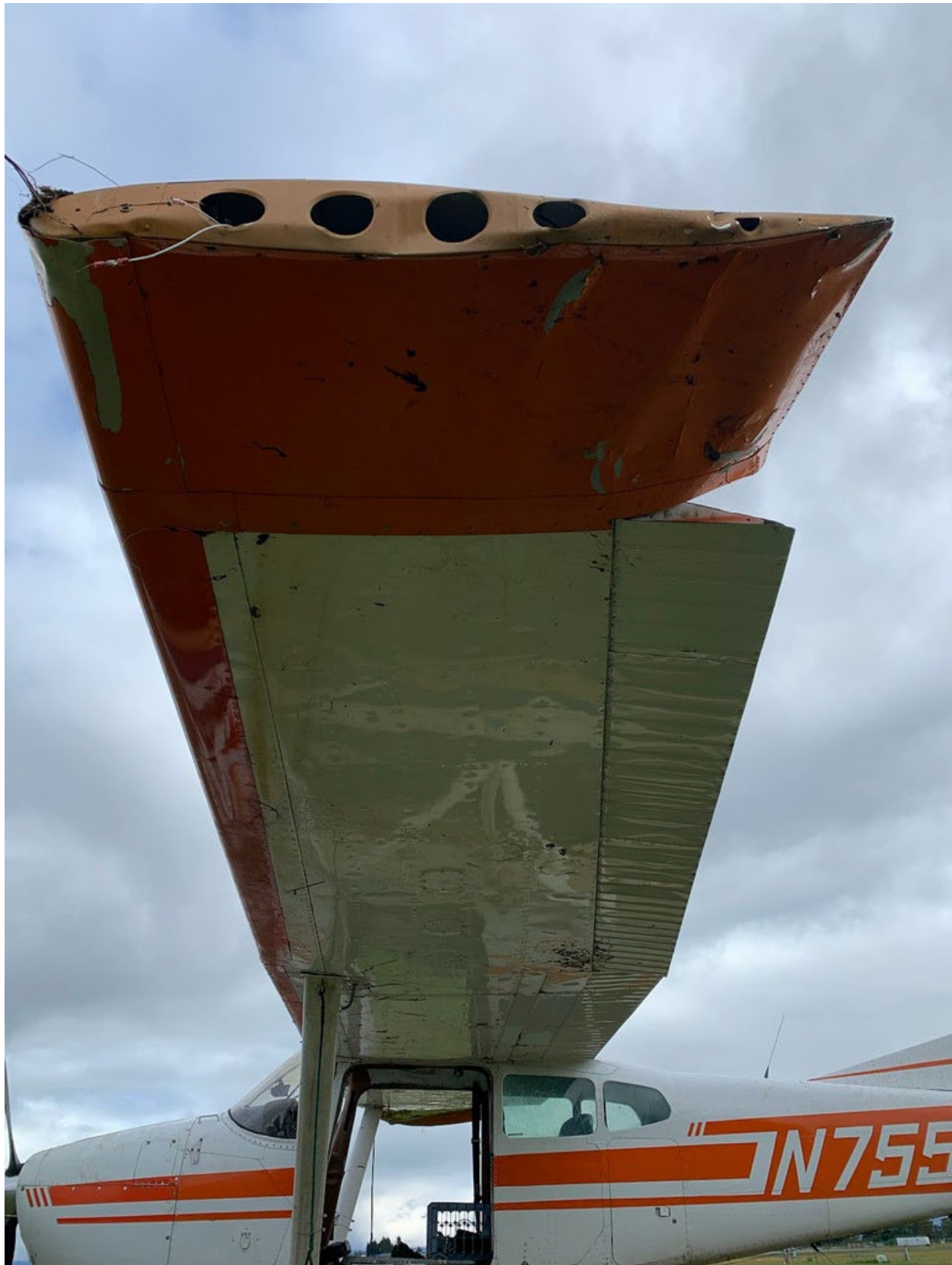
Figure 2 View of damage to the left wing. (Courtesy of FAA)
