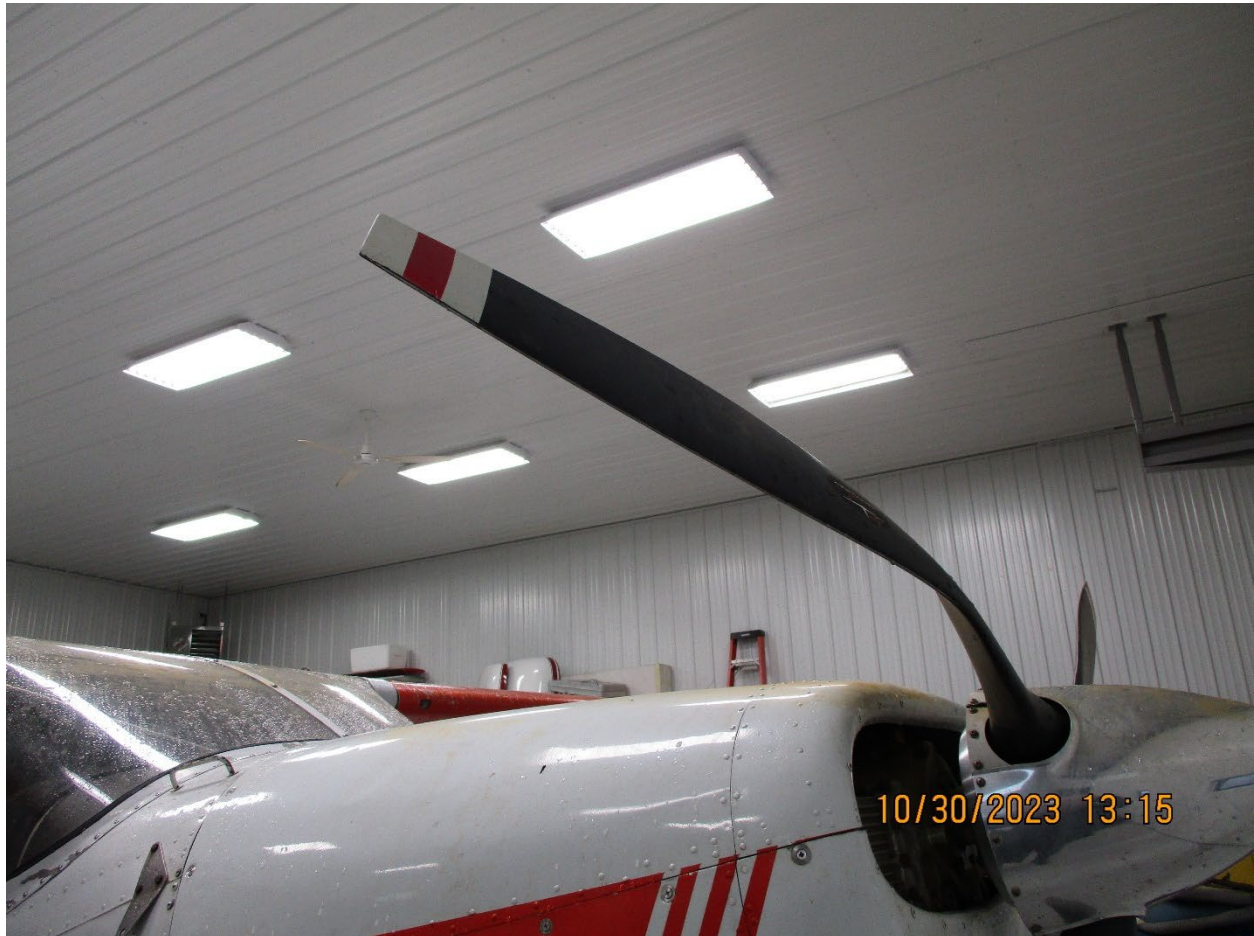
Figure 7 One of the three propeller blades was bent aft. (Courtesy of FAA)
