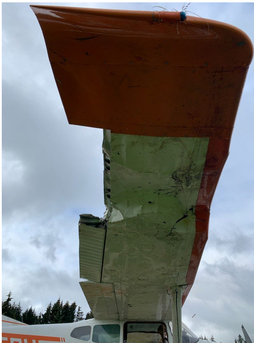
Photograph 3 - View of damage to the right wing (Courtesy of Federal Aviation Administration)
