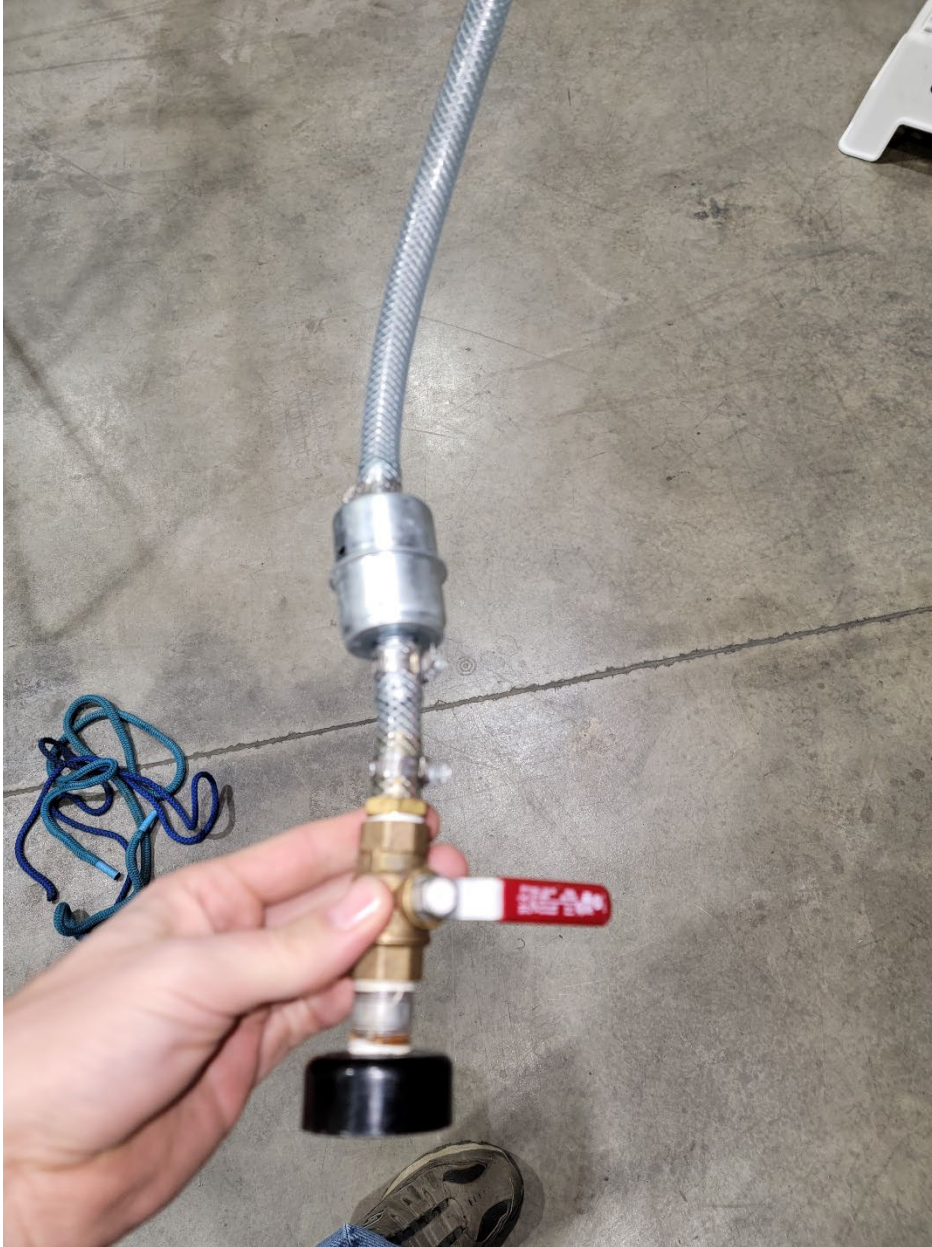
Figure 5. Hose and filter assembly used to transfer fuel from the Swiss fuel bags.
