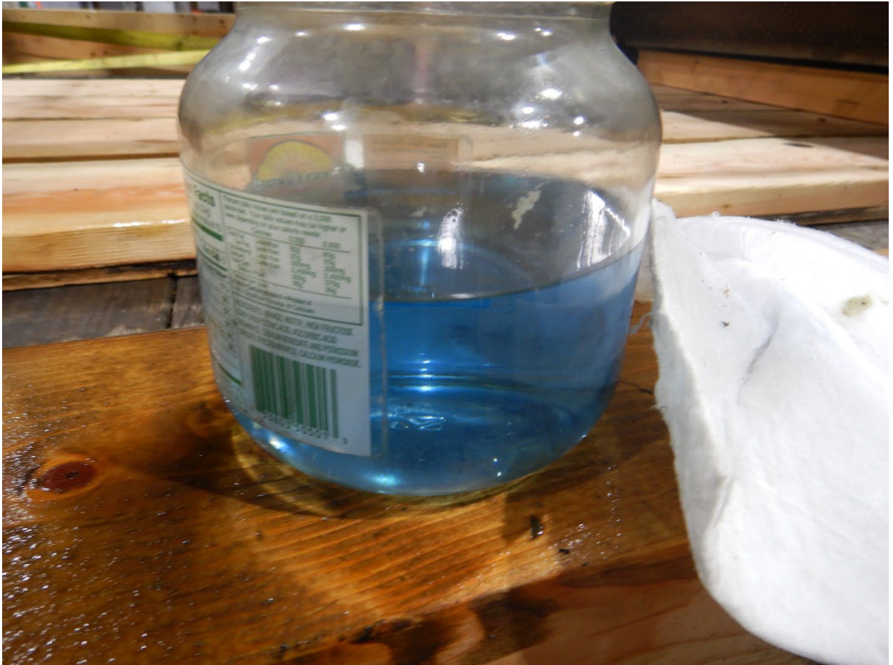
Figure 2. Fuel recovered from the airplane's fuel lines.
