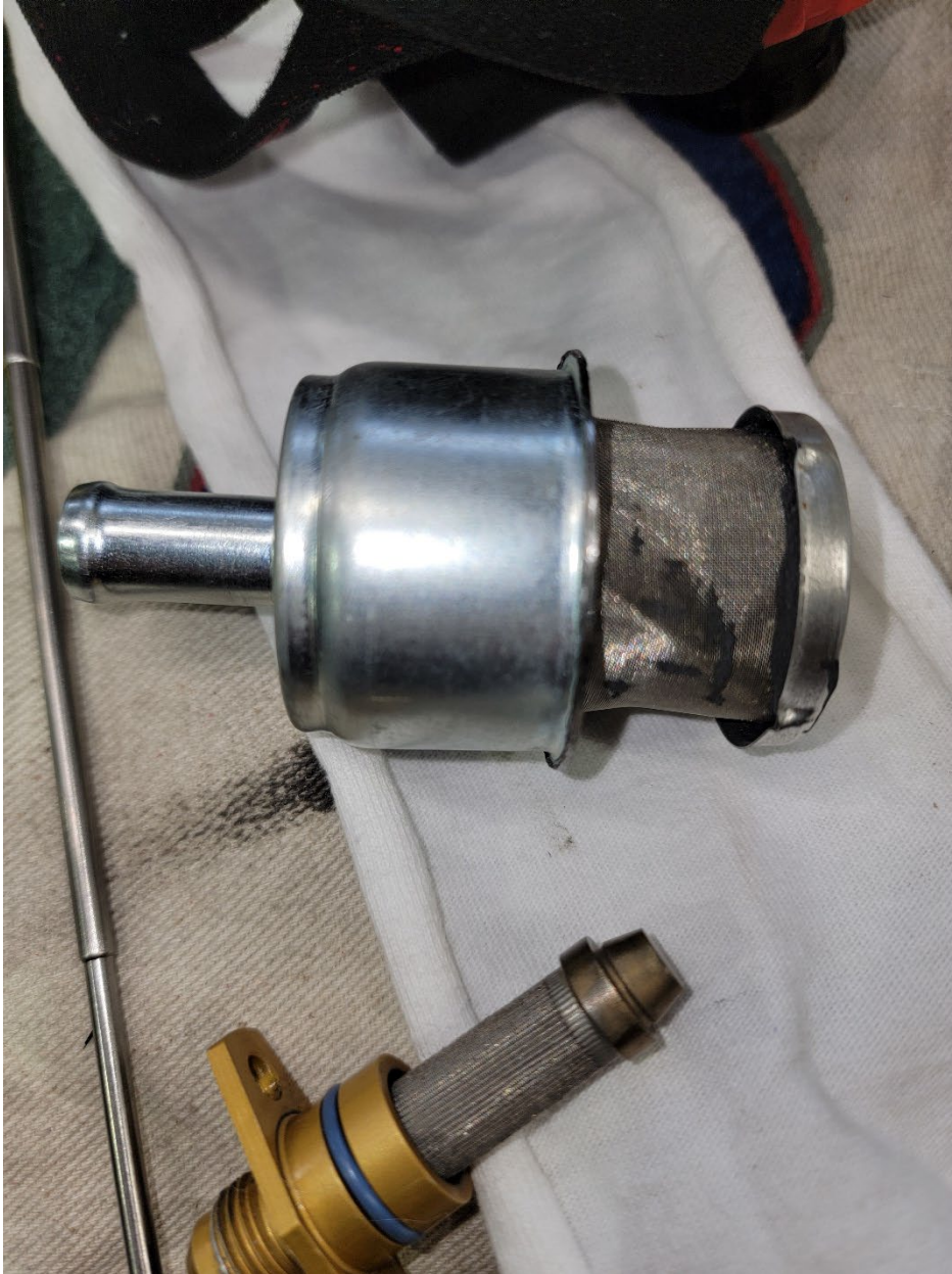
Figure 6. Metal filter screen used when transferring fuel from the Swiss fuel bags into the airplane's fuel tanks.
