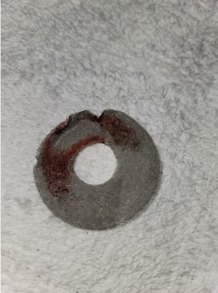
Figure 3. Gascolator screen from accident airplane.
